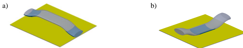
Fig. 7. Rigid joint between the nanocomposite mat and the fabric (a) upper yarn (b) bottom yarn (Geometry scaled)
