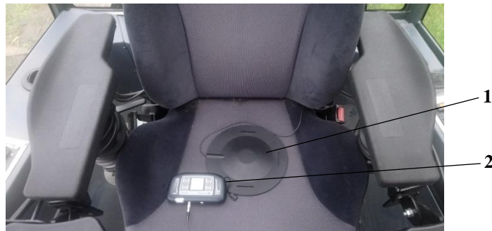
Fig. 2. Whole body vibration measurement instrumentation: 1 – seat pad accelerometer; 2 –Bruel&Kjaer type 4447 human vibration analyser
