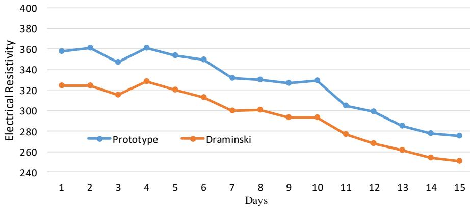
Fig. 4. Prototype and Draminski Mastitis Detector data correlation for cow No.14 during 15 days
