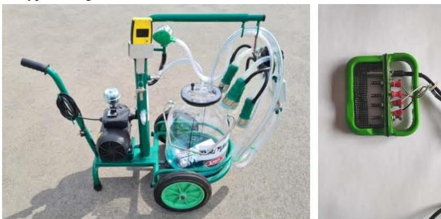
**Fig. 2. Small milking machine used for IoT prototype (on left) and a sensor module (on right)**
