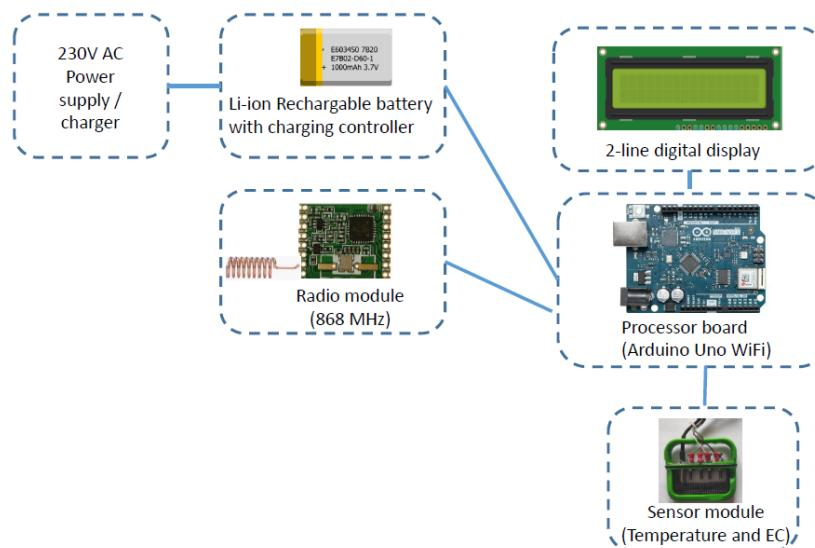
Fig. 1. Flowchart of IoT based prototype
