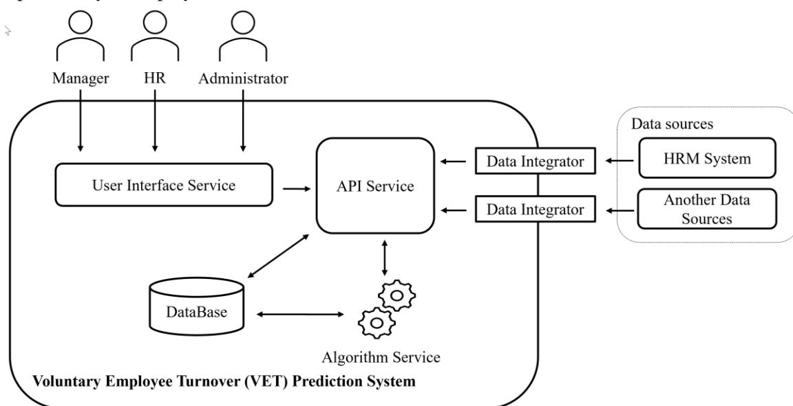
Fig. 1. Common architecture of VET prediction
