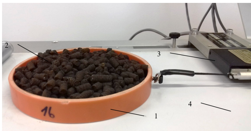
Fig. 1. View of organic granulated manure pellets particle-wall friction force and friction coefficients determination device: 1 – ring; 2 – pellets; 3 – force measuring element; 4 – metal plate
