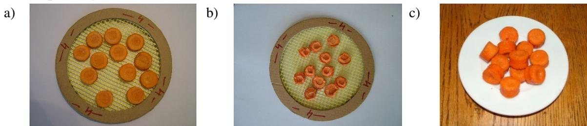
Fig. 1. Carrot sample: a – before drying; b – after drying; c – after rehydration
