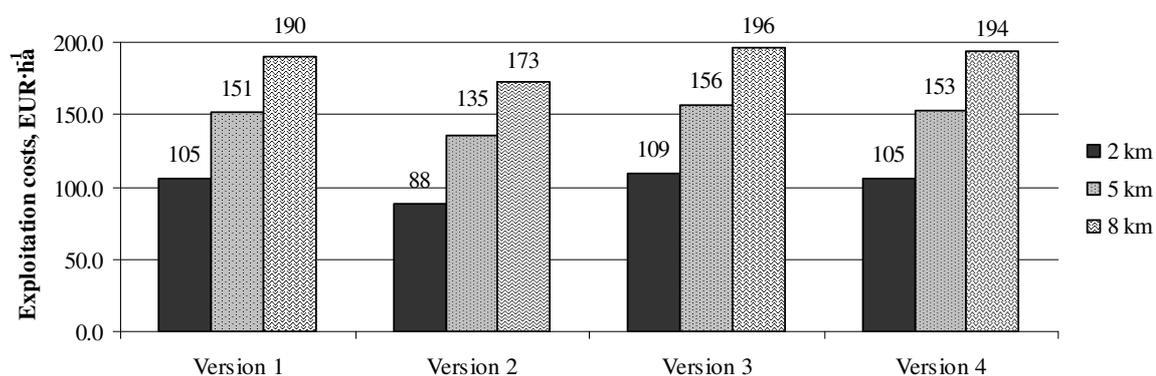
Fig. 3. Costs of liquid manure transportation, spreading and incorporation depending on the technological version and the distance of transportation
