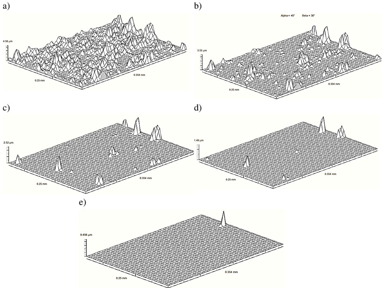
Fig. 7. **Surface cut offs on different levels:** a – surface cut off along midline; b – surface cut off  $1\sigma$  above midline; c – surface cut off  $2\sigma$  above midline; d – surface cut off  $3\sigma$  above midline; e – surface cut off  $4\sigma$  above midline
