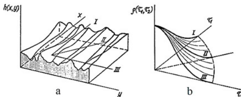
Fig. 1. Schematic depiction of irregular surface roughness (a) and corresponding standardised correlation function (b)
