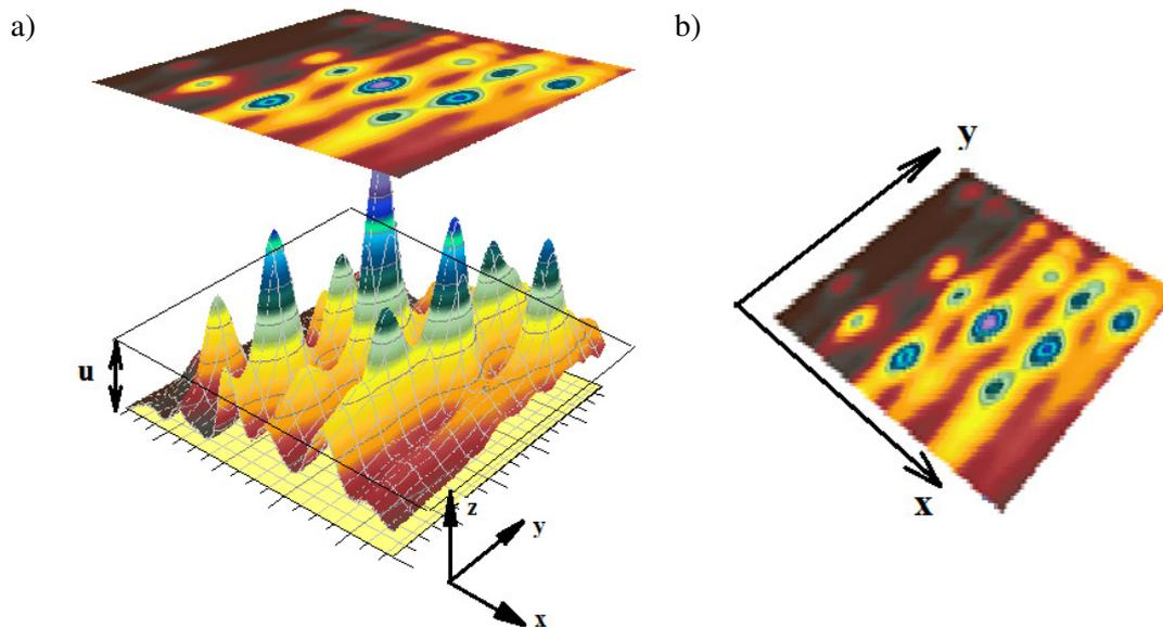
Fig. 2. **Graphic representation of number of surface peaks [2]:** a – 3D surface cut off at level  $u$ ; b – cut off of surface peaks at level  $u$ , view from above
