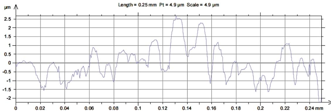
Fig. 6. Profile towards y-axis (along the shortest sample's side)
