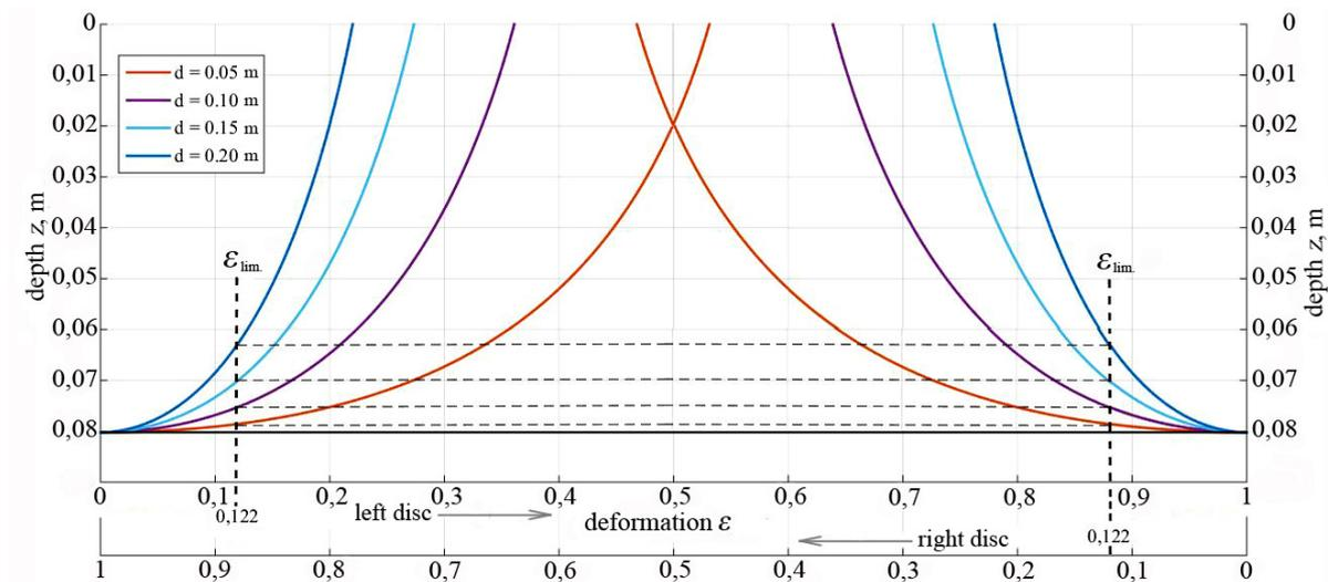
Fig. 8. Diagrams of soil deformation at tilling depth of  $a = 0.08$  m and at different values of distance between disks  $d$  (for fixed values of disc radius  $R = 0.25$  m and inclination angles of  $\gamma = 6^\circ$ )
