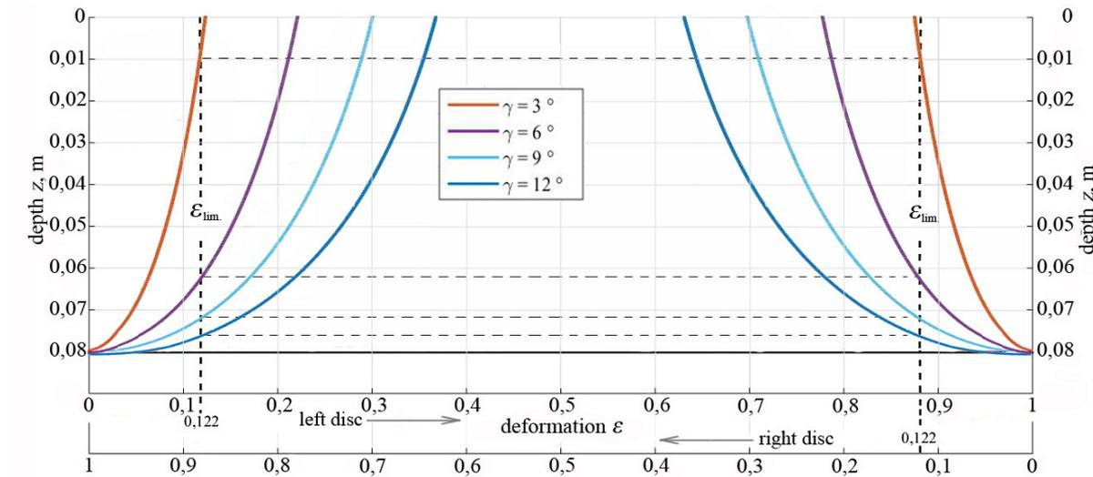
Fig. 9. Diagrams of soil deformation at tilling depth of  $a = 0.08$  m and different values of disc inclination angle of  $\gamma$  (for fixed values of disc radius  $R = 0.25$  m and distance between discs  $d = 0.2$  m)
