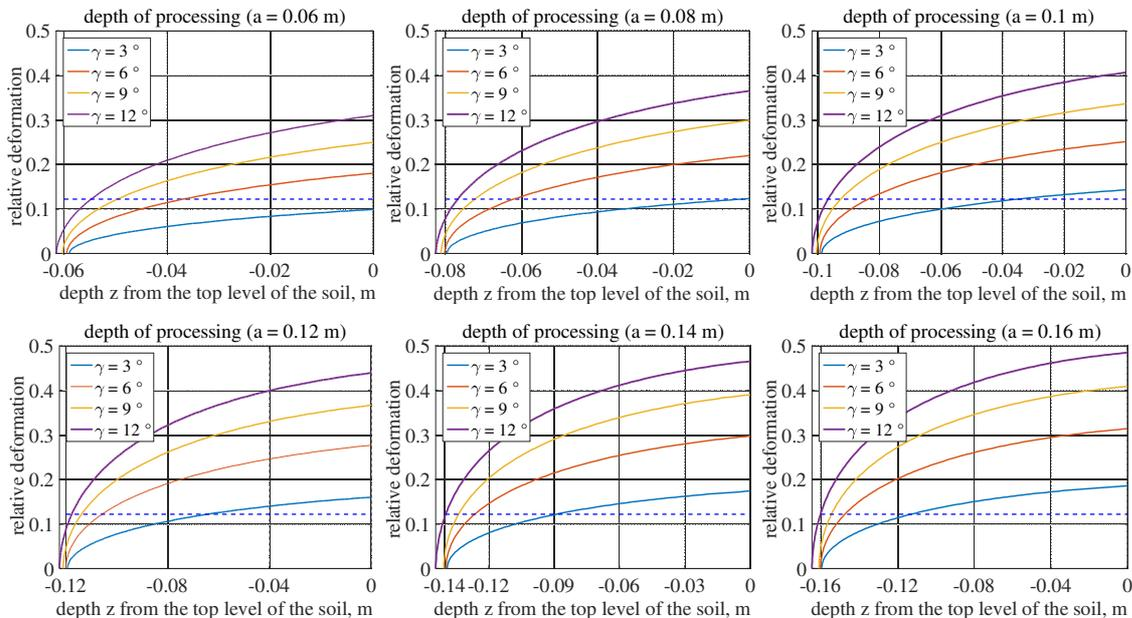
**Fig. 6. Dependence of relative soil deformation  $\epsilon$  from  $z$  coordinate at different values of tillage depth and the disc inclination angle of  $\gamma$  (for fixed values of disc radius  $R = 0.25$  m and the distance between discs  $d = 0.2$  m; ----- the limit value of relative soil deformation)**
