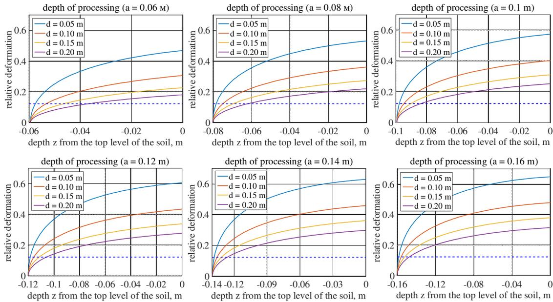
**Fig. 5. Dependence of relative soil deformation  $\epsilon$  from  $z$  coordinate at different values of tillage depth and the distance between discs  $d$  (for fixed values of disc radius  $R = 0.25$  m and the disc inclination angle of  $\gamma = 6^\circ$ ; ----- the limit value of relative soil deformation)**
