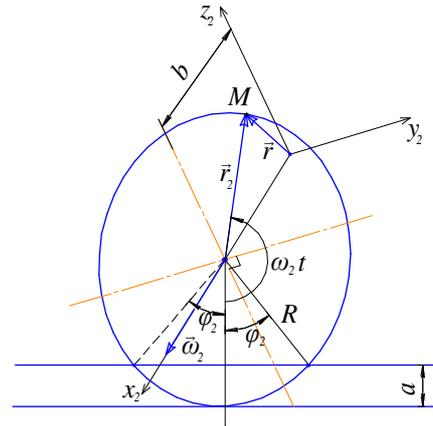
Fig. 4. Diagram for determining the formula of the disc edge circumference in the system  $(x_2, y_2, z_2)$  in cylindrical coordinates
