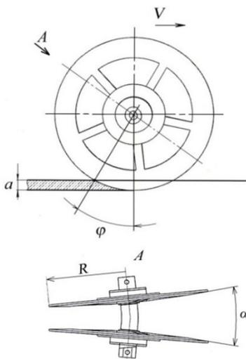
Fig. 1. Section of a disc cultivator
