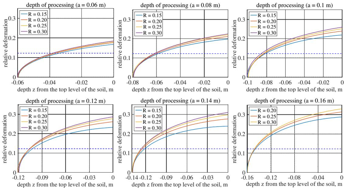
Fig. 7. Dependence of relative soil deformation  $\varepsilon$  from  $z$  coordinate at different values of tillage depth and distance between discs  $d$  (for fixed values of disc radius  $R = 0.25$  m and the disc inclination angle of  $\gamma = 6^\circ$ ; ----- the limit value of relative soil deformation)
