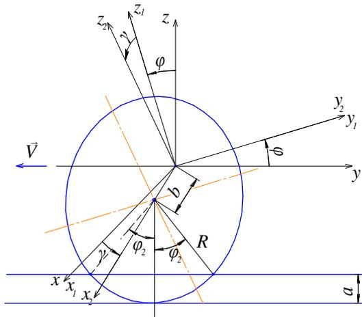
Fig. 3. Transformation of disc coordinate points, in passing to the coordinate axis, related to the aggregate frame  $(x, y, z)$
