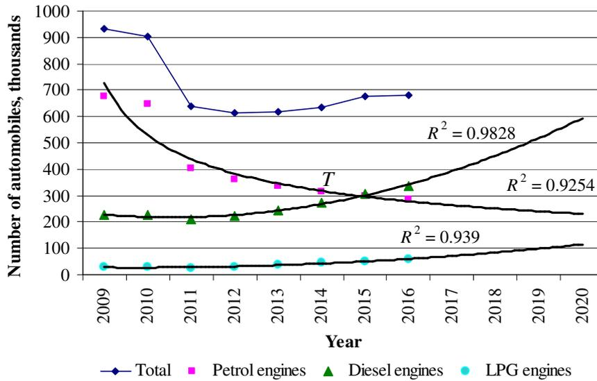
Fig. 1. Changes in the distribution of cars and light lorries by engine type
