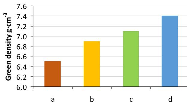
Fig. 6. Change in the pressing density depending on the specific energy of discharge 0.8; 0.9; 1.0 and 1.2 kJ·cm<sup>-3</sup>
