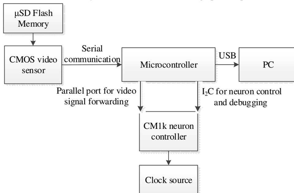
Fig. 2. Sensor structure
