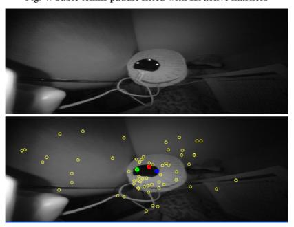
Fig. 5. Identification of markers in captured image from Leap Motion stereo cameras
