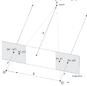
Fig. 8. Marker positioning in 3D space using stereoscopic projections
