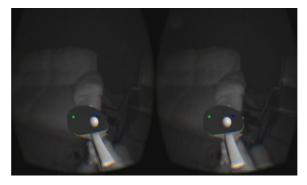
Fig. 3. Table tennis paddle and a virtual ball in augmented reality using active infrared markers
