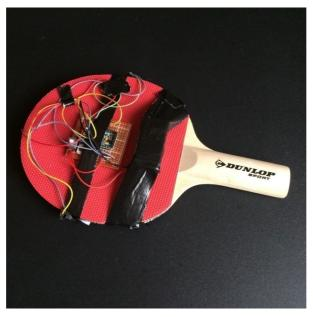
Fig. 4. Table tennis paddle fitted with IR active markers
