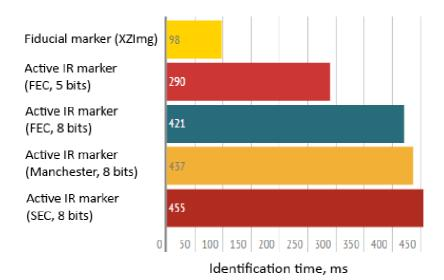
Fig. 9. Performance of active IR markers with different types of error correction
