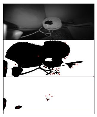
Fig. 7. Binary filter with thresholdranges for tracking LED markers
