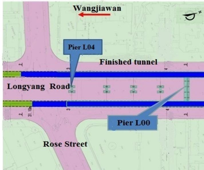
Fig. 3. BIM simulation pier locations and tunnel construction
