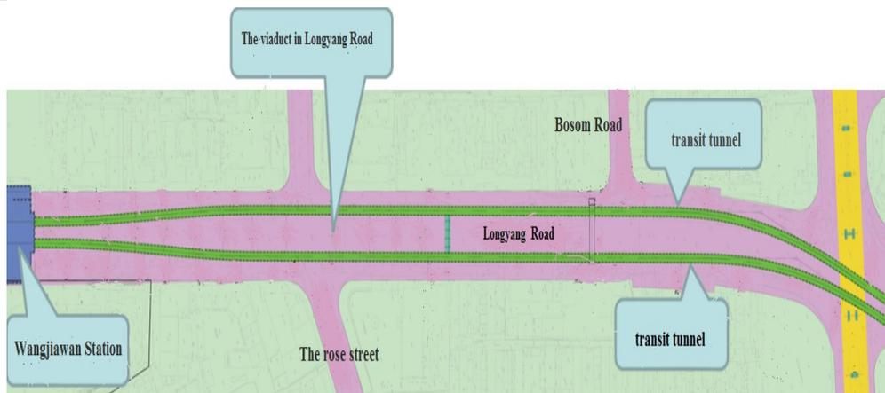
**Fig. 1. Schematics of Wangjiawan Station and Zongguan concerning Longyang Road station intervals overpass plane location**
