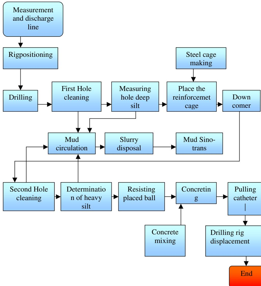
Fig. 5. Impact Drill Hole Pile Construction flow chart
