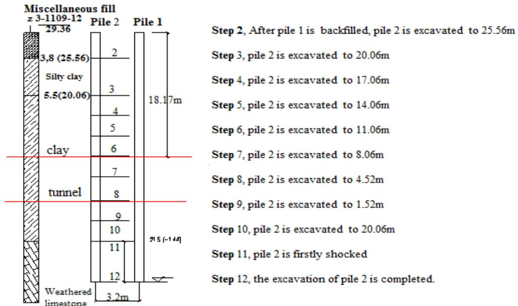
Fig. 7. Pile schematic construction process simulations
