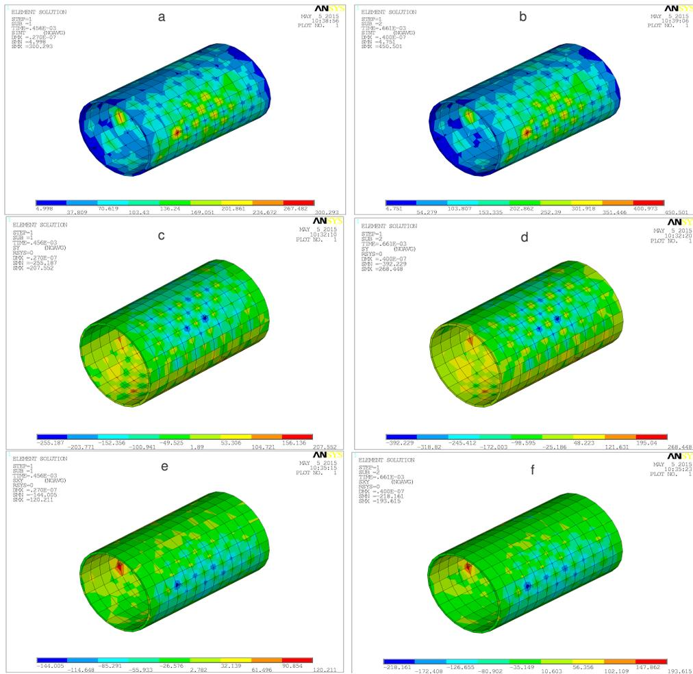
**Fig. 8. After construction is completed pile 1 Lining moment cloud (a), After completion of construction of pile lining 2 moment cloud (b), After construction is completed pile 1 shear lining cloud (c), After completion of construction of pile lining 2 shear cloud (d), 1 pile shaft lining after construction contour plots (e), After completion of construction of pile lining 2 axis contour plots (f)**
