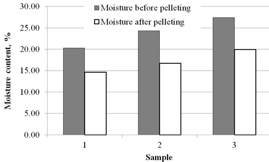
Fig. 5. Moisture content before and after granulation
