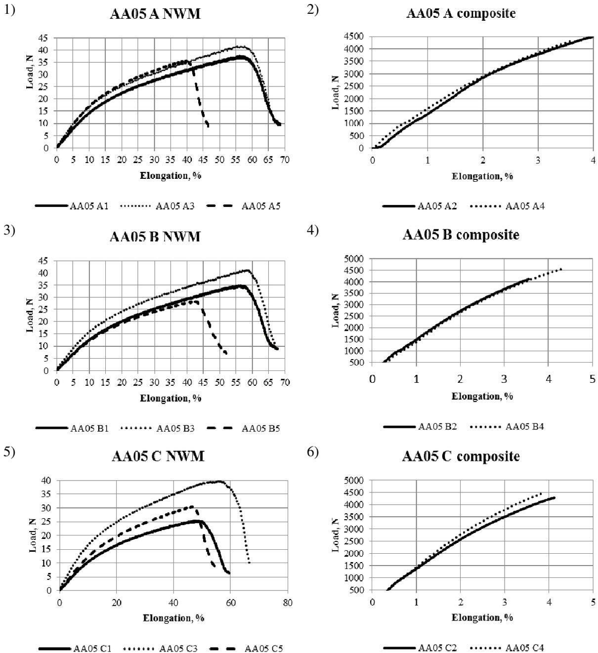
Fig. 3. Diagrams showing relationship between NWM and composite material strip elongation and the applied load: 1 – NWM sample A; 2 – composite sample A; 3 – NWM sample B; 4 – composite sample B; 5 – NWM sample C; 6 – composite sample C
