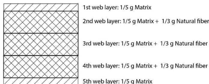
Fig. 1. Schematic structure of nonwoven material
