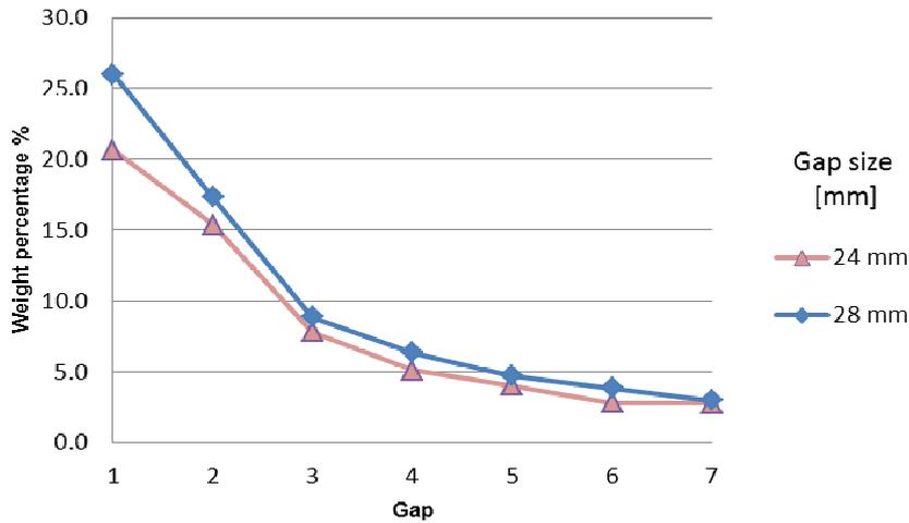
**Fig. 4. Weight percentage of the hop matter fallen through the separate gaps with rollers of 82.5 mm in diameter and rotation frequency of 0.67 s<sup>-1</sup>**
