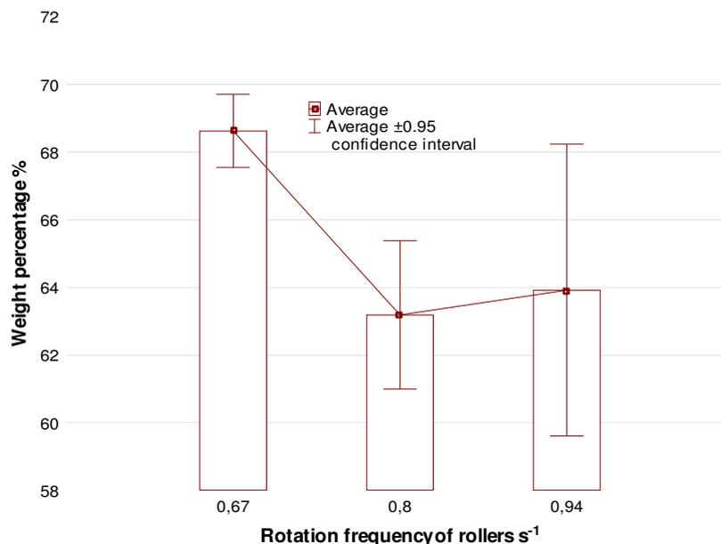
Fig. 8. Weight percentage of leaves and small-sized impurities in the waste with rollers of 82.5 mm in diameter, gap of 24 mm and three rotation frequencies
