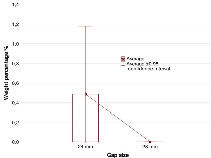
Fig. 6. Weight percentage of hop cones in the waste with rollers of 82.5 mm in diameter and rotation frequency of  $0.67 \text{ s}^{-1}$
