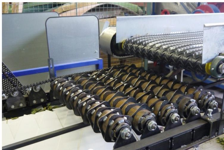
Fig. 2. Laboratory roller conveyor with rollers fitted with welded collars
