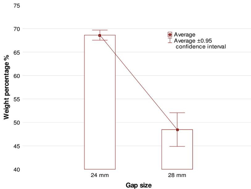
**Fig. 5. Weight percentage of the leaves and small-sized impurities in the waste with rollers of 82.5 mm in diameter and rotation frequency of 0.67 s<sup>-1</sup>**
