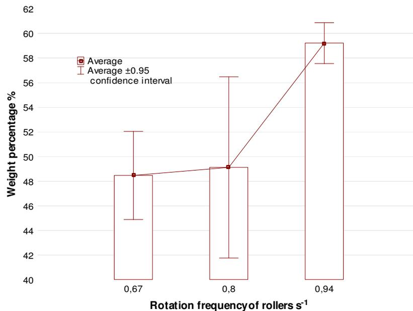
Fig. 7. Weight percentage of leaves and small-sized impurities in the waste with rollers of 82.5 mm in diameter, gap of 28 mm and three rotation frequencies
