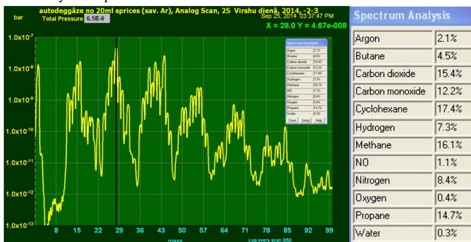
Fig. 7. Spectrum analysis of the gas, graph (left) and consistence of the gas obtained from AHP (right)
