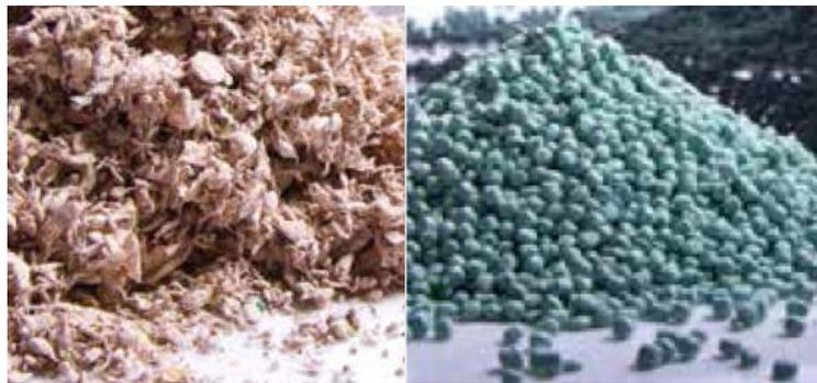
Fig. 1. **Fibres obtained from recycled AHPs (left) and plastic pellets obtained from recycled AHPs (right)**
