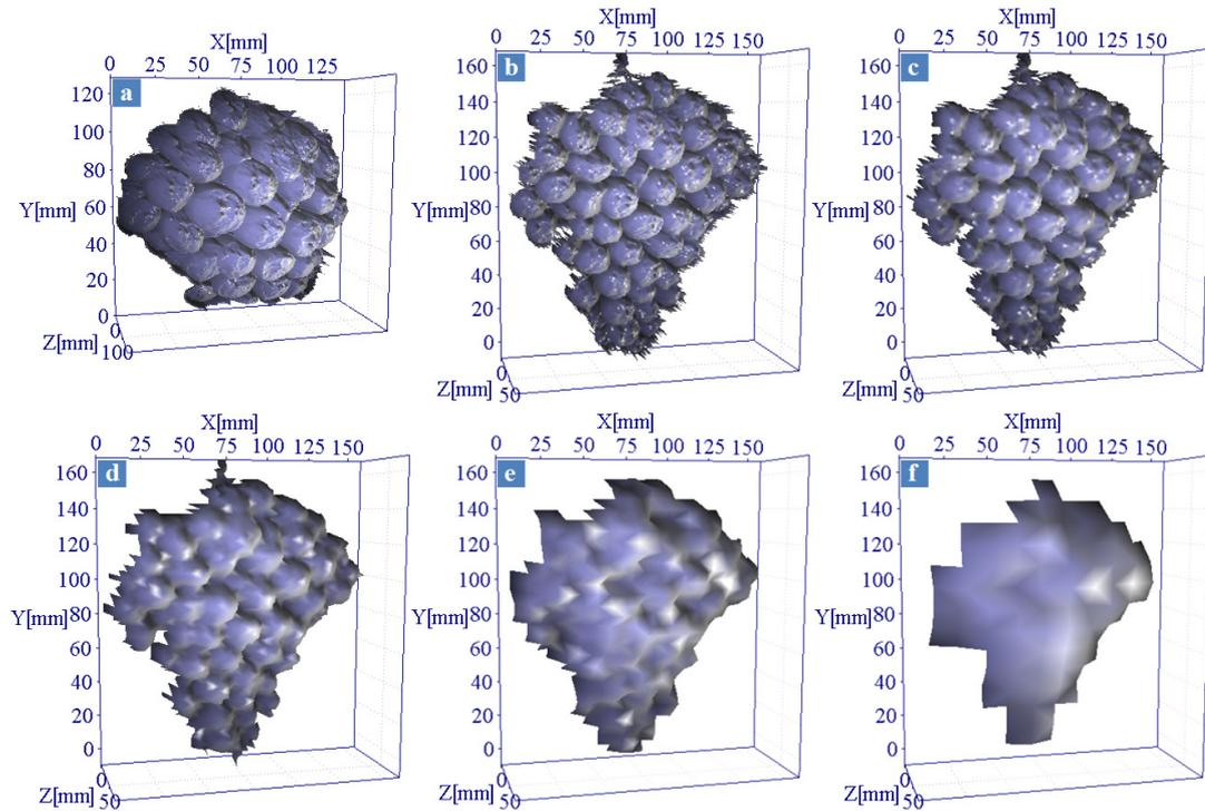
Fig. 5. 3D rendering of a grape cluster scanned from the bottom at a 0.8 m distance (a) and from the side at increasing distances: 0.8 m (b), 1.2 m (c), 2.0 m (d), 4.0 m (e) and 8.0 m (f)
