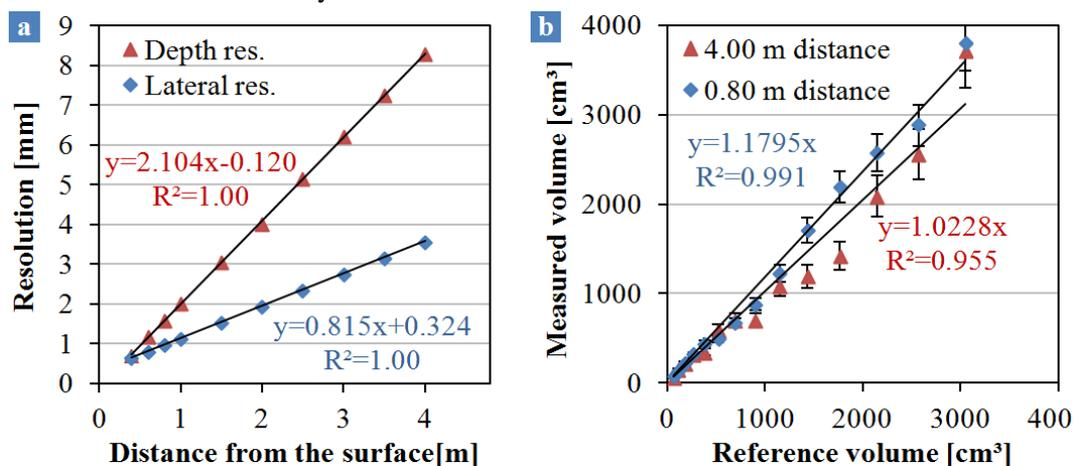
Fig. 4. (a) Lateral and depth resolutions and (b) measured as a function of reference volumes at different relative distances of the sensor from the target surface. Error bars represent standard deviations of five repeated measurements
