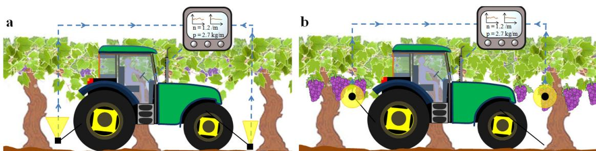
Fig. 2. Two possible configurations with the three-dimensional sensor measuring from the bottom (a) or from the side (b)
