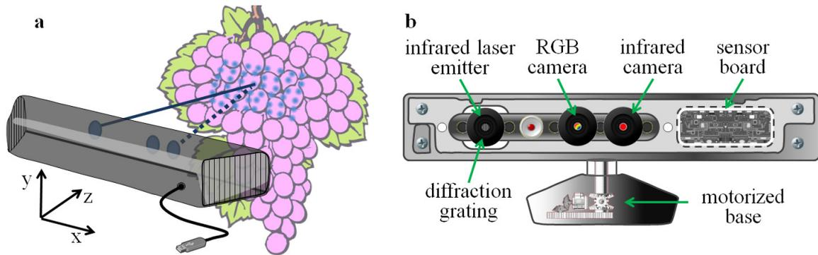
Fig. 1. Kinect 3D sensing is based on a triangulation principle (a); schematic view of the Kinect sensor with infrared (IR) projector, IR and RGB cameras localization (b)
