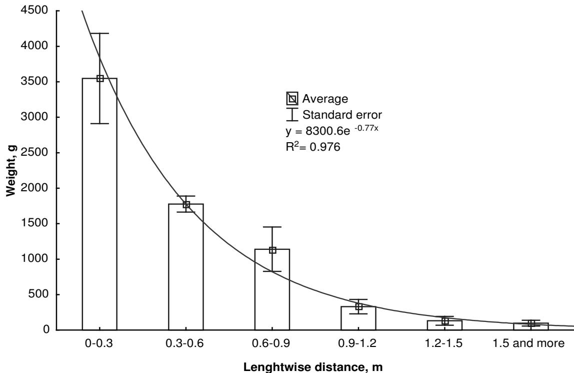
Fig. 1. Average values of particle translocation in a lengthwise direction for reduction technology
