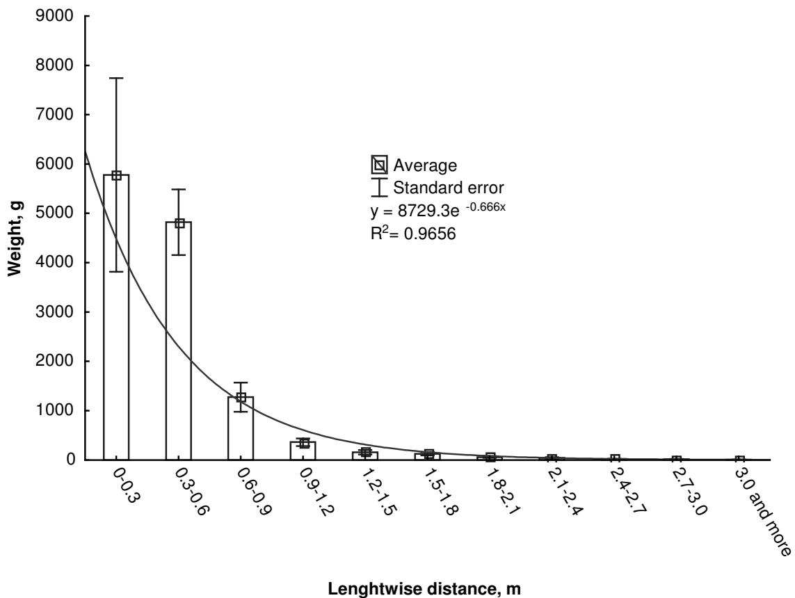
Fig. 3. Average values of particle translocation in a lengthwise direction for conventional technology
