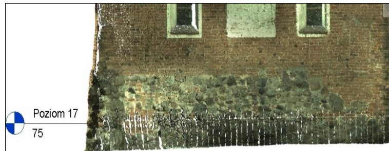
Fig. 5. Horizontal contour running across the cloud at 75 cm
