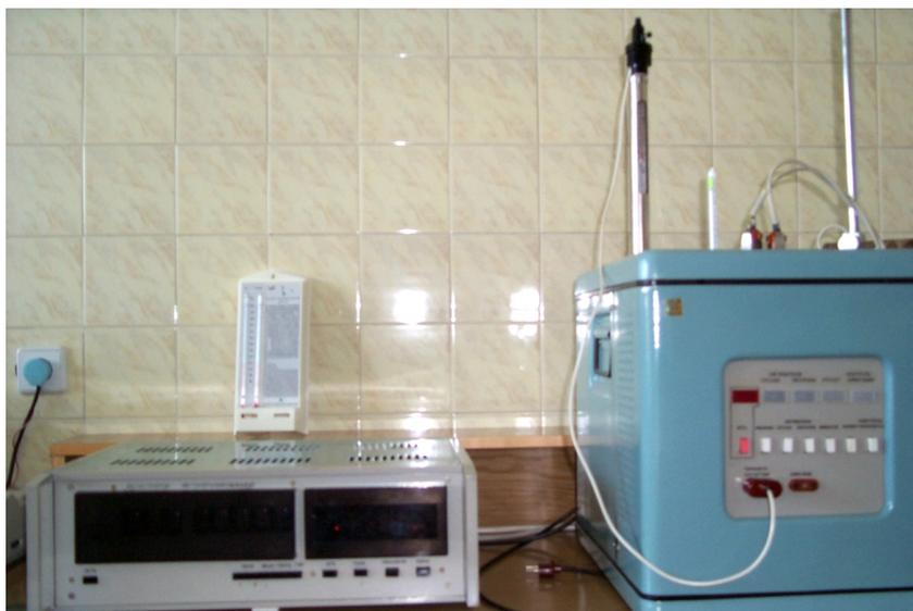
Fig. 1. General view of calorimeter V-08 MA with temperature registrar ABL 646.00.00
