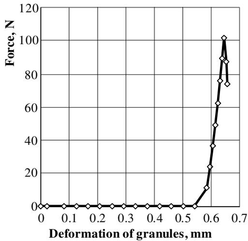
Fig. 3. Deformation (mm) and disintegration force (N) of granulated Kieserite granules
