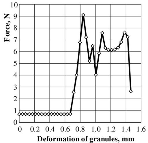
Fig. 4. Deformation (mm) and disintegration force (N) of granulated Serpentine larger-size granules
