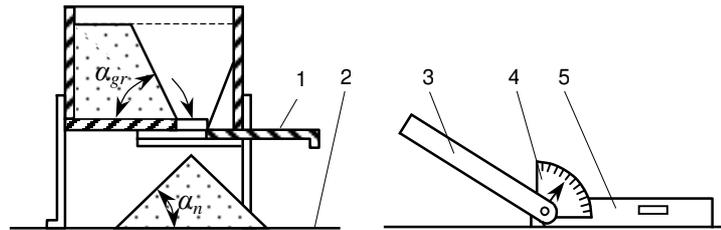
Fig. 1. Scheme of determination equipment of natural slope and fall angles: 1 – damper; 2 – horizontal surface; 3 – turning ruler; 4 – protractor; 5 – ruler with level
