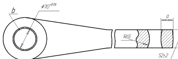
Fig. 3. **Central suspension rod:** a – upper bridge lug; b – lower lug bushing
