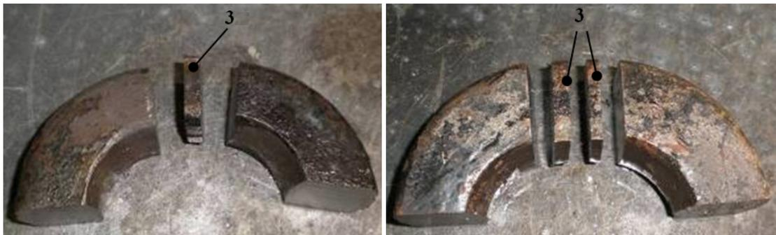
Fig. 7. **Rod of the central spring suspension:** 3 – cross sectional slice of rod with wear (left);
