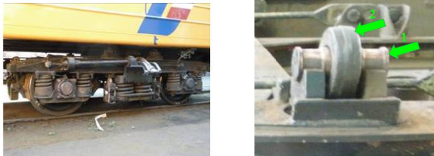
Fig. 1. **Suspension parts:** 1 – roller; 2 – central suspension rod
