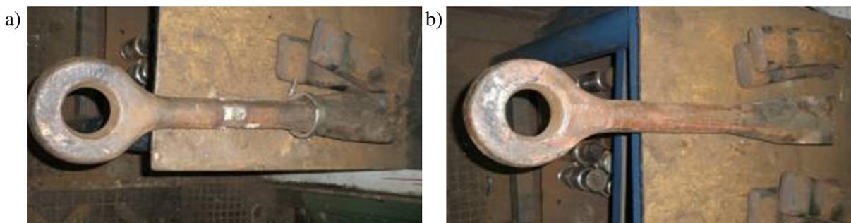
Fig.5. **Central suspension rod:** a – new; b – with wear
