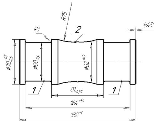
Fig. 2. **Roller:** 1 – roller bearing surface; 2 – roller central part
