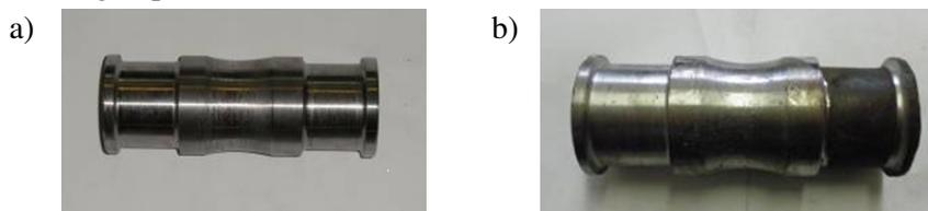
Fig. 4. **Roller:** a – new; b – repaired
