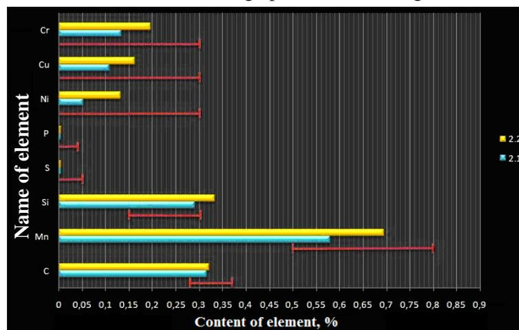
Fig. 8. Graphical representation of the results of the samples 2.1., 2.2 chemical analyses
