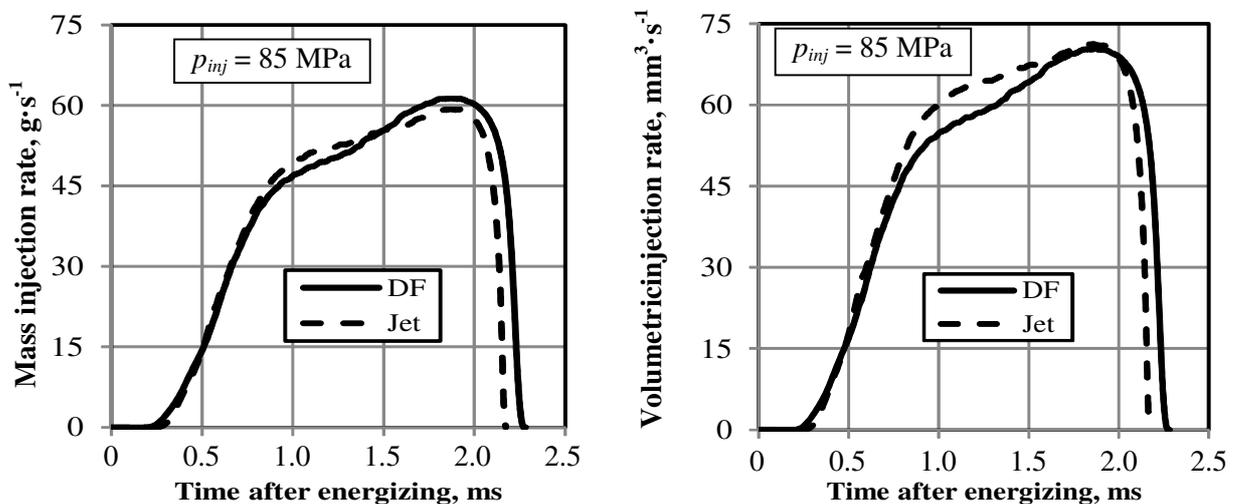
Fig.5. Simulated diesel and jet fuel mass and volumetric injection rate
