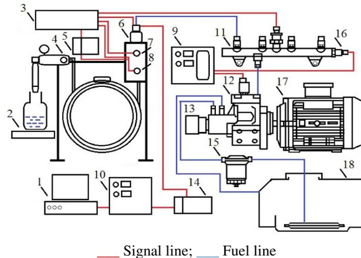
Fig. 1. **Scheme of the fuel injection rate test rig:** 1 – PC; 2 – electronic scale; 3 – data acquisition module; 4, 8 – pressure sensors; 5 – charge amplifier; 6 – injector; 7 – temperature sensor; 9 – fuel pressure control unit; 10 – injector driver; 11 – fuel rail; 12 – HP pump; 13 – pressure regulator; 14 – NI 9161 chassis; 15 – fuel filter; 16 – rail pressure sensor; 17 – EC motor; 18 – fuel tank
