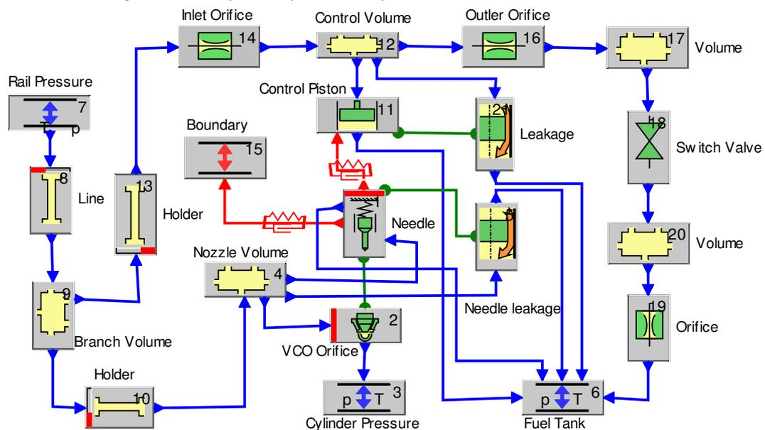
Fig. 2. **Boost-Hydsim model of the common rail injector:** injector type CRIN2-16, nozzle type DLLA 140P1790
