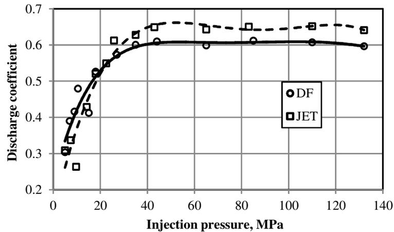
Fig. 4. Discharge coefficient versus injection pressure for diesel and jet fuels
