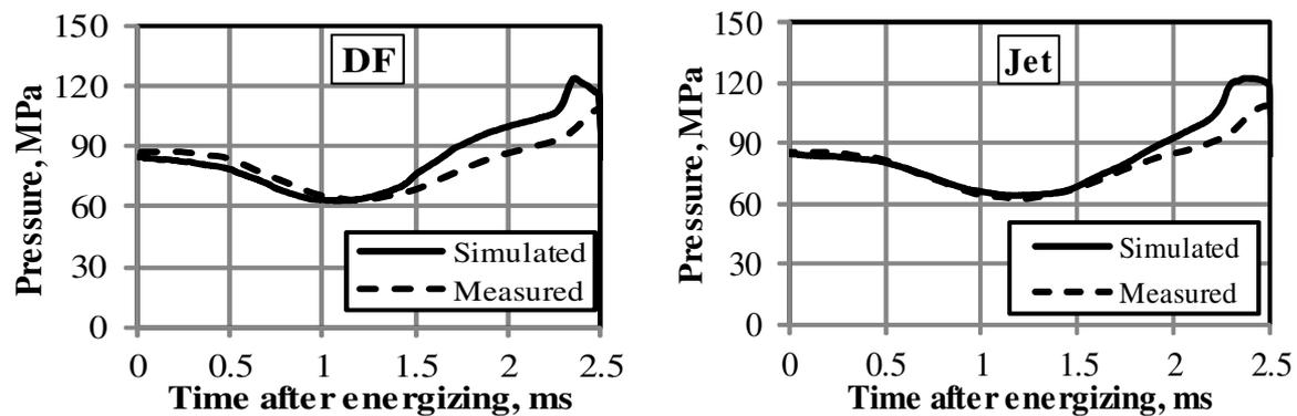
Fig.6. Measured and simulated pressure in injection duct
