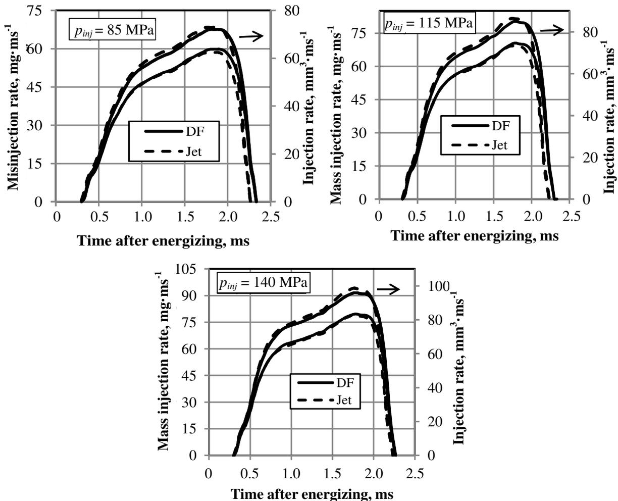
Fig. 3. Effect of the injection pressure and fuel type on the injection rate: back pressure 4.0 MPa, energizing time 1.3 ms
