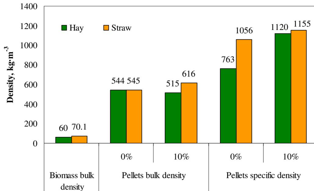
Fig. 1. Density of biomass and pellets from hay and straw with or without addition of calcium carbonate
