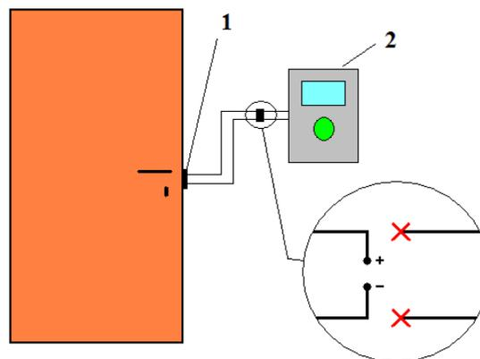
Fig. 2. **Sabotage of the system with direct control:** 1 – electrical lock; 2 – reader
