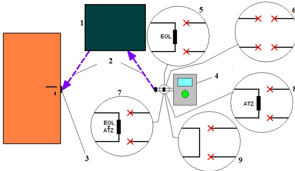
Fig. 3. Sabotage of the system with I&HAS: 1 – I&HAS; 2 – inaccessible wiring; 3 – electrical lock; 4 – reader; 5 – with EOL and without ATZ or with EOL ATZ N.O.; 6 – without EOL and ATZ or with EOL and without ATZ N.C.; 7 – with EOL and ATZ N.C.; 8 – without EOL and with ATZ N.C.; 9 – without EOL and with ATZ or without EOL and without ATZ N.O.
