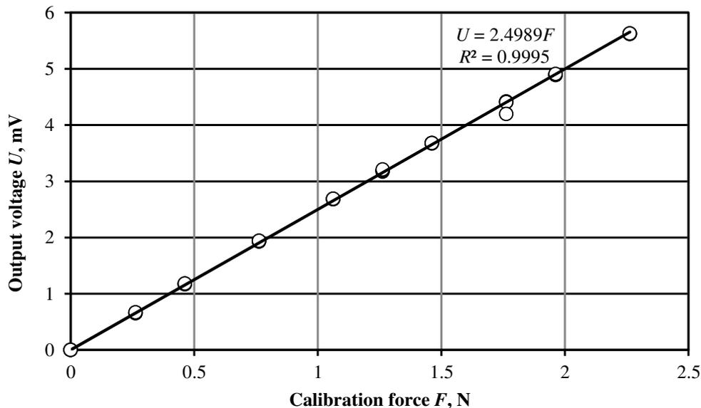
Fig. 5. Calibration curve of power sensor
