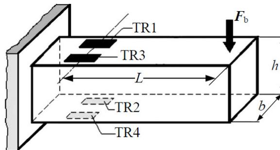
Fig. 4. **Force sensor structure:** TR1, TR2, TR3, TR4 – resistance strain gauges;  $L$  – distance between the center of attachment of resistance strain gauge to the location where the force is applied;  $F_b$  – applied force;  $h$  – height of the metal plate;  $b$  – width of the metal plate
