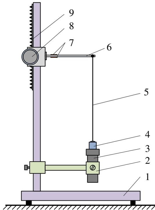
Fig. 3. **Scheme of the experimental facility:** 1 – stanchion; 2 – binding; 3 – plunger liner; 4 – plunger; 5 – flexible string; 6 – power sensor; 7 – resistance strain gauges; 8 – hand wheel; 9 – rack
