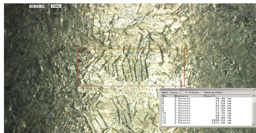
Fig. 4. Identification of the relative width of cracks in a sample bent at a  $R_{out} = 3.32 \text{ mm}$  (50x magnification)
