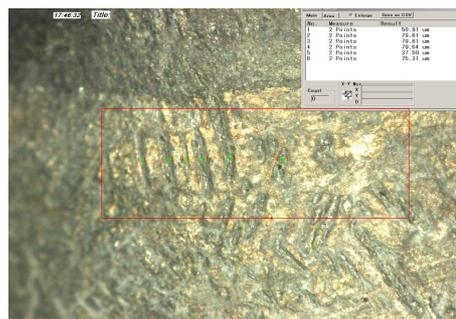
Fig. 7. Sample folded at an outside bend radius of 3.32 mm (100x magnification)
