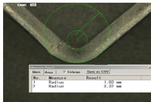
Fig. 2. Bend radius measurements for Sample No. 20
