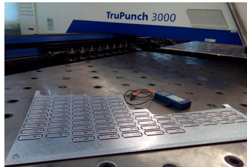
Fig. 1. Sample placement in a sheet and a devise for measuring zinc layer thickness
