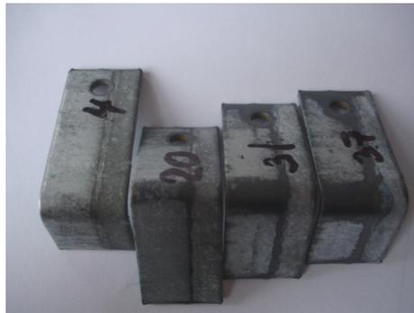
Fig. 6. Corrosion signs on the samples (sample No.4 was exposed to the acid for 24 h, No.20 – for 48 h, No.31 – for 72 h and No.37 – for 96 h)
