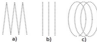
Fig. 3. **Scan patterns:** a – sinusoidal scan pattern; b – parallel scan lines; c – elliptical scan pattern
