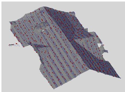
Fig. 6. Roof and trace of LiDAR points
