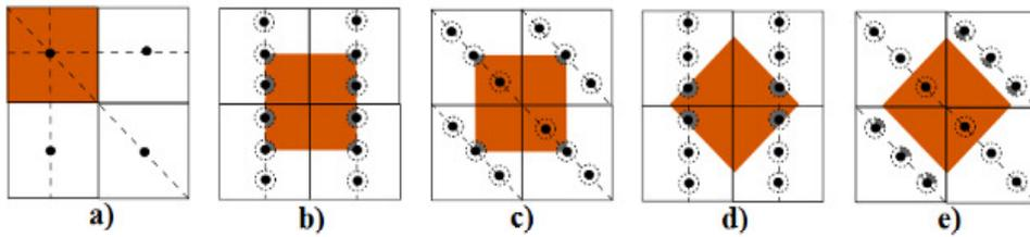
Fig. 9. **Object location patterns:** a – best case for detection; b – average case with vertical scanning trace; c – average case with diagonal scanning trace; d – worst case with vertical scanning trace; e – worst case with diagonal scanning trace
