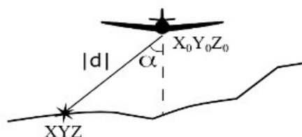
Fig. 1. Scheme of airborne laser scanning
