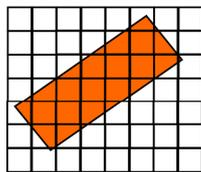
Fig. 4. Building projected on grid of ground samples
