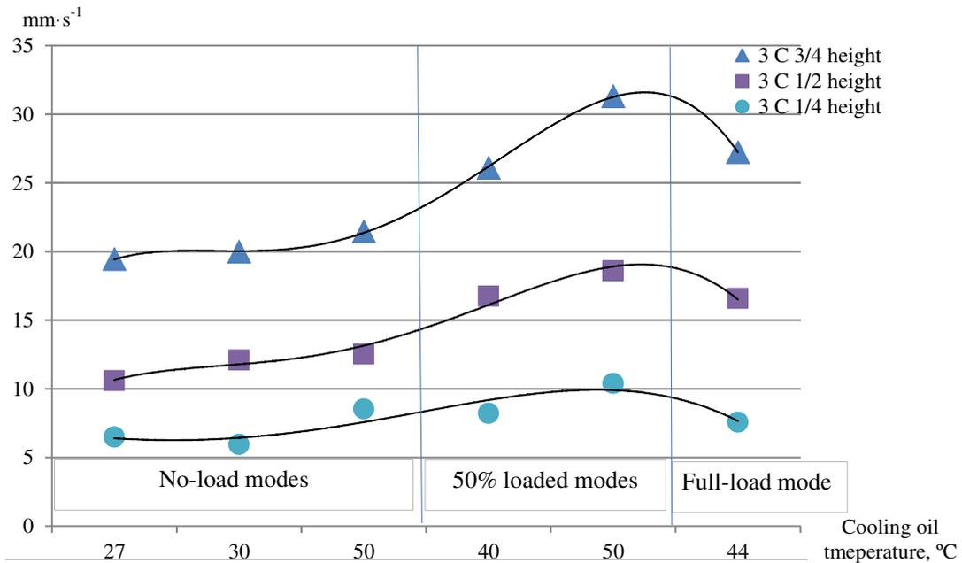
Fig. 1. Vibration velocity rise in loaded modes for the 3<sup>rd</sup> column (HV side)
