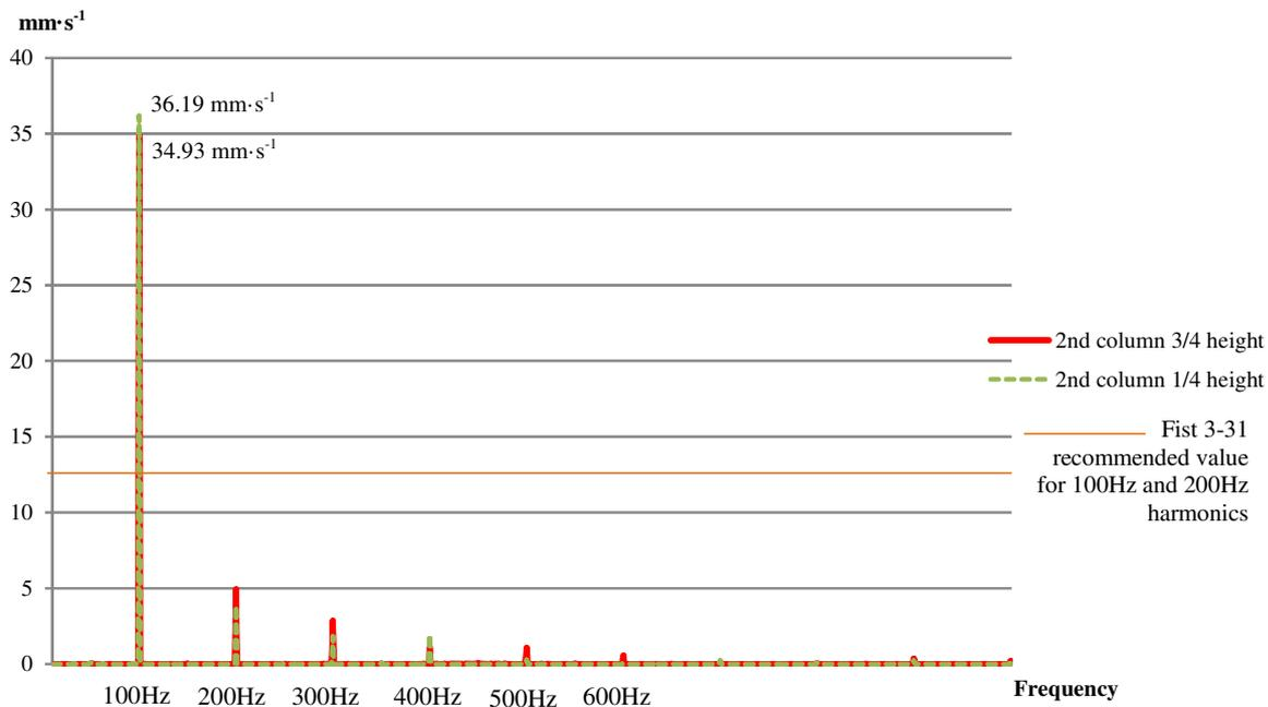
Fig. 3. Vibration velocity spectrum in no-load mode, shell side
