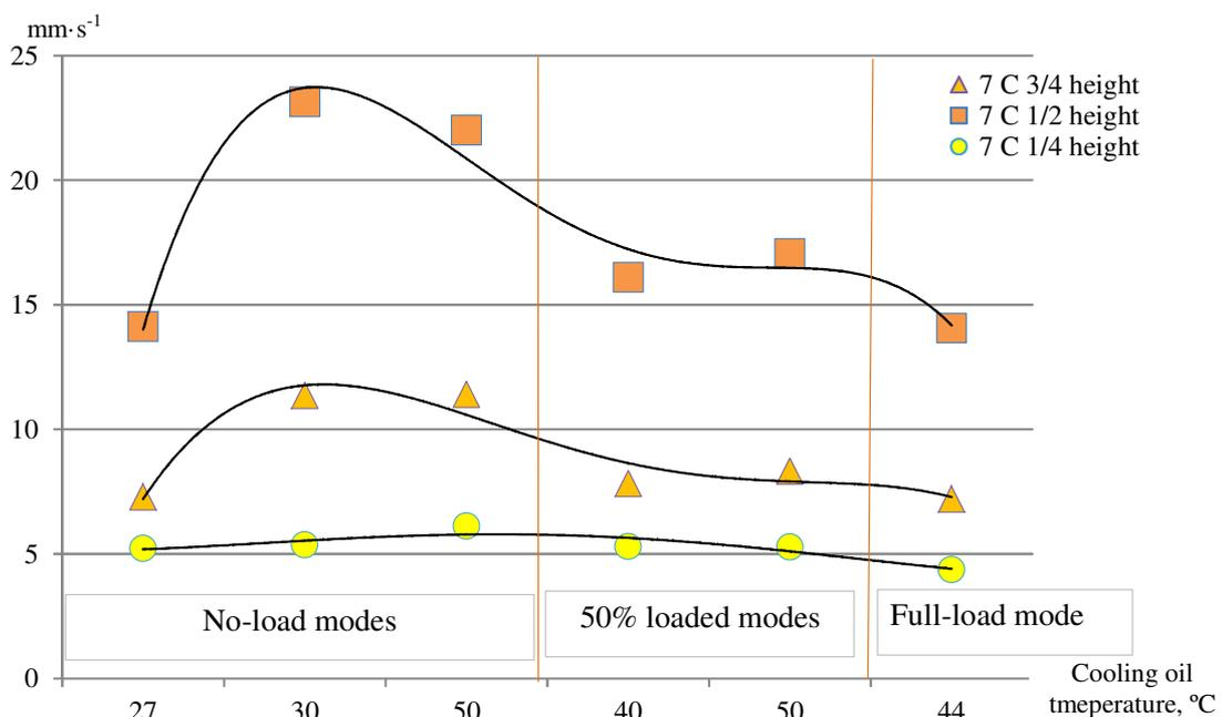
Fig. 2. Vibration velocity drop in loaded modes for the 7<sup>th</sup> column (HV side)
