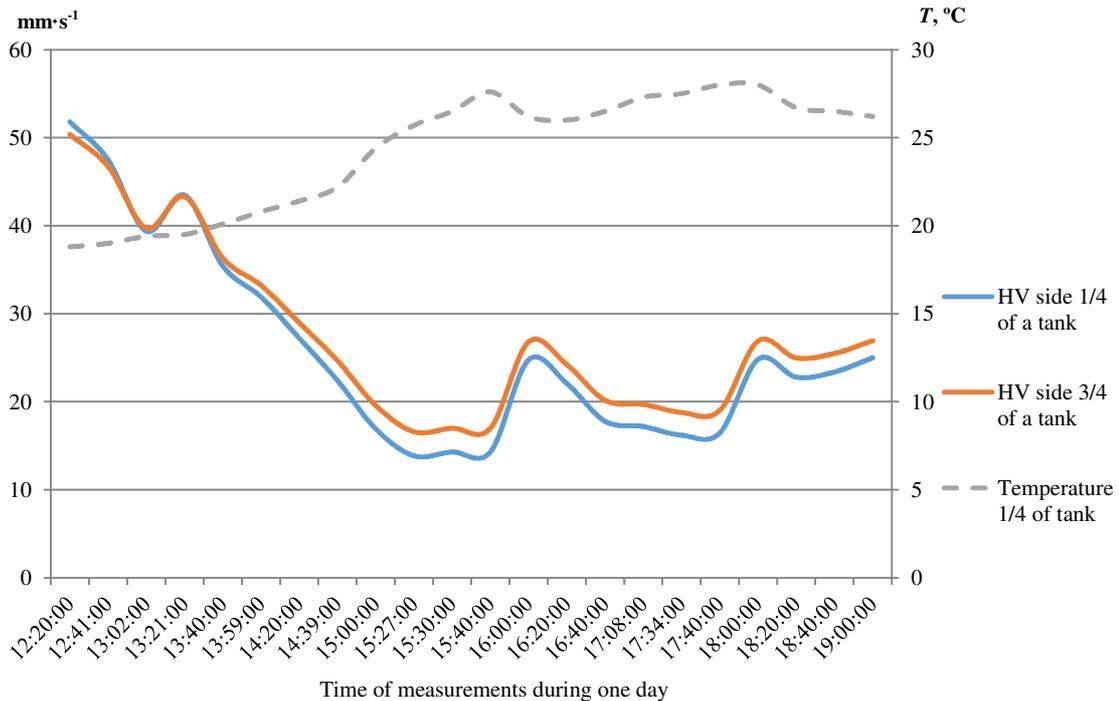
Fig. 4. Correlation of transformer tank vibration and cooling oil temperature
