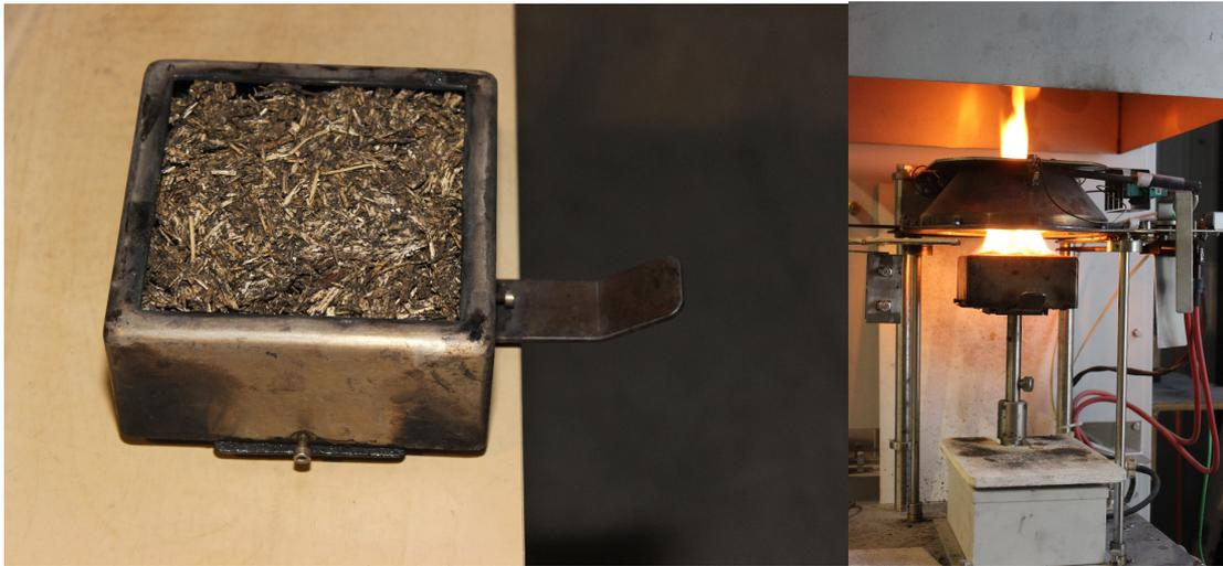
Fig. 1. Sapropele hemp shive mixture test in the conic calorimeter
