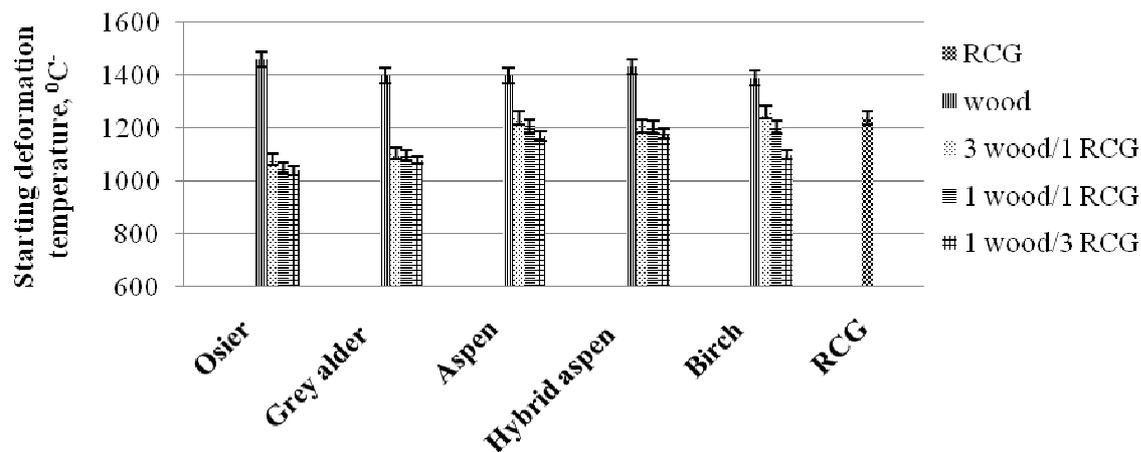
Fig. 4. Starting deformation temperature of reed canary grass and timber pellets
