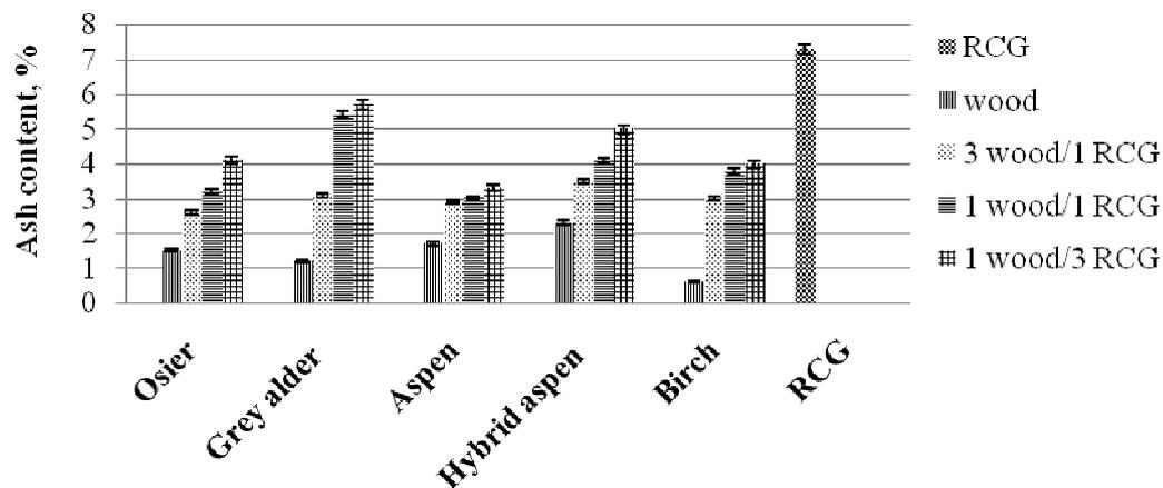
Fig. 3. Ash content in reed canary grass and timber pellets
