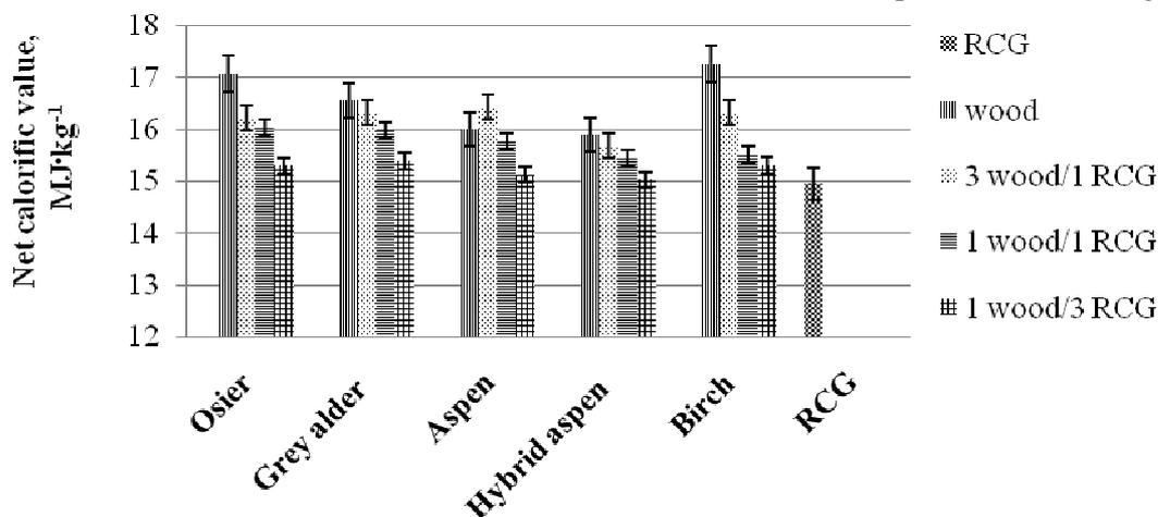
Fig. 1. Net calorific value of reed canary grass and timber pellets, moisture content: osier – 7 %; gray alder – 7.7 %; poplar – 7.4 %; hybrid aspen – 8.5 %; birch – 8.5 %; reed canary grass – 8.5 %
