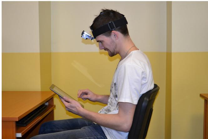
Fig. 2. Testing setup with iPad 2 and GoPro Black Edition Hero4 action camera
