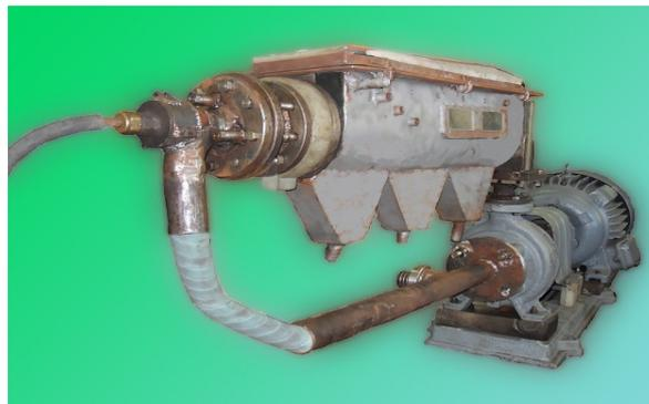
Fig. 2. Appearance of vortex cavitator with water jacket
