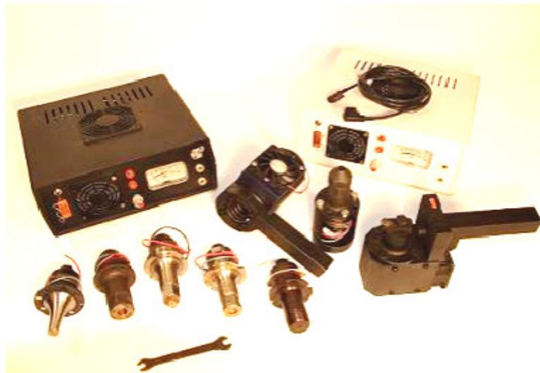
Fig. 5. Devices for auto-resonant ultrasonic turning and smoothing
