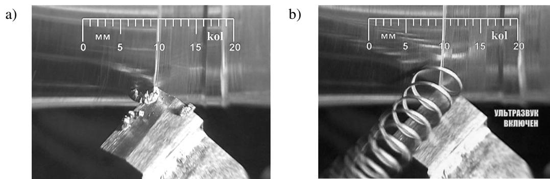
Fig. 2. Chips in: a – traditional process; b – ultrasonic turning
