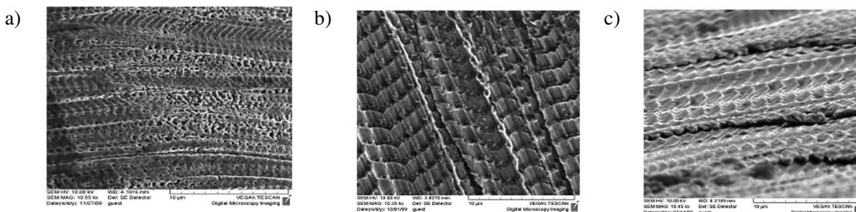
Fig. 4. **Reinforcing nanostructures:** a – copper; b – brass; c – steel
