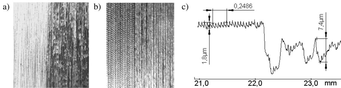
Fig. 3. **Hardened steel:** a, b – treated surfaces; c – example of profilogram
