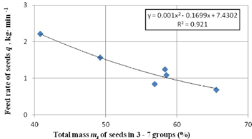
Fig. 2. Dependency of distribution of white mustard seeds into fractions 3-7 on feed rate of seeds  $q$  to inclined plane
