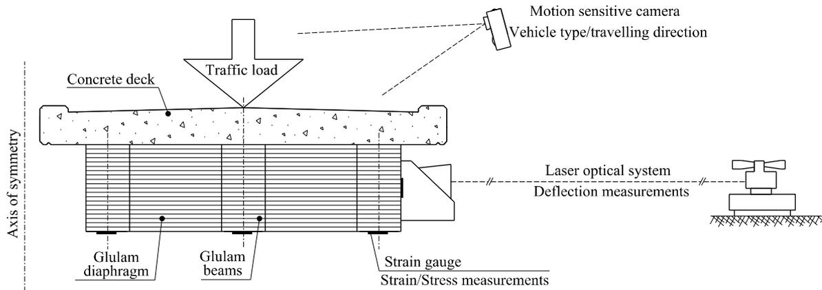
Fig. 1. Layout of the measurement system
