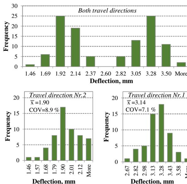
Fig. 5. Deflection measurements (decomposed by directions)
