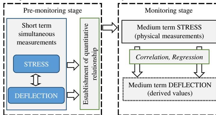
Fig. 2. Principal scheme of monitoring
