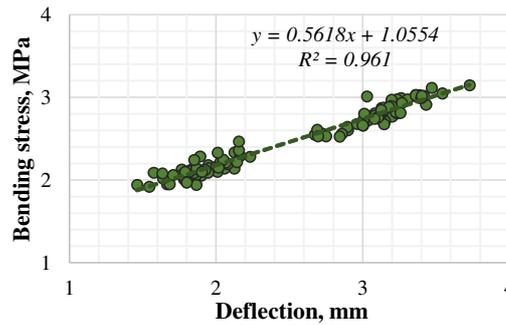
Fig. 4. Bending stress and deflection data pairs.
