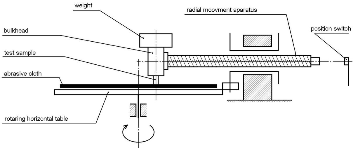
Fig. 1. Test of resistance to abrasive cloth [10; 12]
