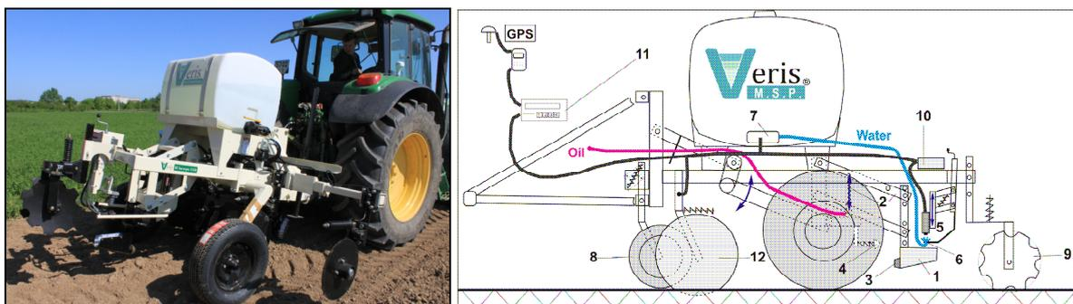
Fig. 1. Veris MSP machine with Soil pH Manager system: 1 – scoop; 2 – mechanism of scoop lifting; 3 – adapter; 4 – hog; 5 – pH sensors; 6 – water supply with nozzles; 7 – water tank; 8 – plant residues removal; 9 – furrow filling hoes; 10 – controller; 11 – data recorder; 12 – sensor of soil electrical conductivity
