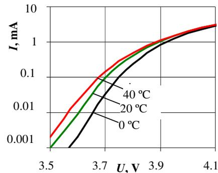
Fig. 10. V/A characteristics of the optoelectronic converter
