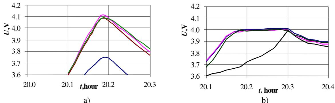
Fig. 3. **Voltages of four cells at the end of the charge cycle:** a) without balancer; b) with balancer
