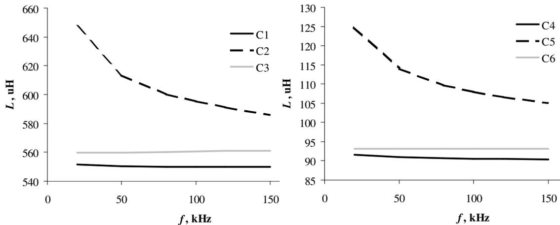
Fig. 3. Inductance  $L$  of coils in relation to frequency
