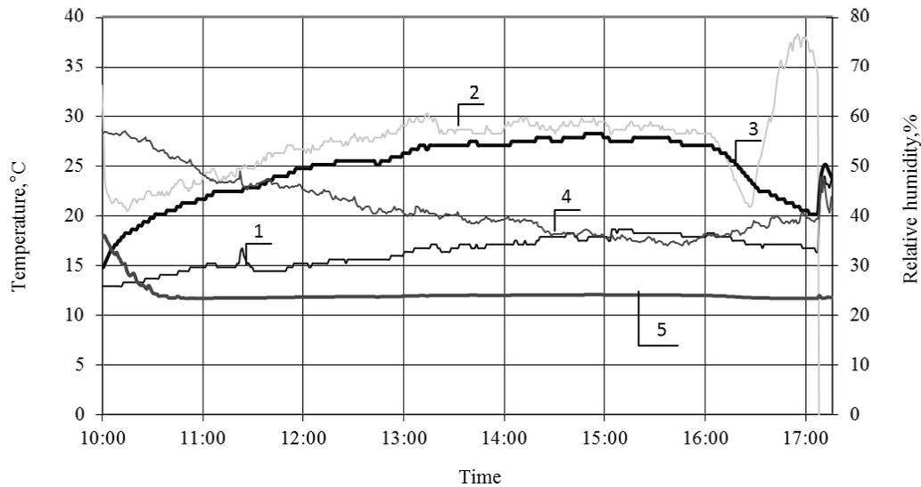
**Fig. 4. Hemp desiccation parameter characteristic graph using the heated air without the solar radiation energy concentrator:** 1 – ambient air temperature; 2 – ambient air relative humidity; 3 – outflow air temperature; 4 – temperature inside the hemp roll; 5 – relative humidity inside the hemp roll
