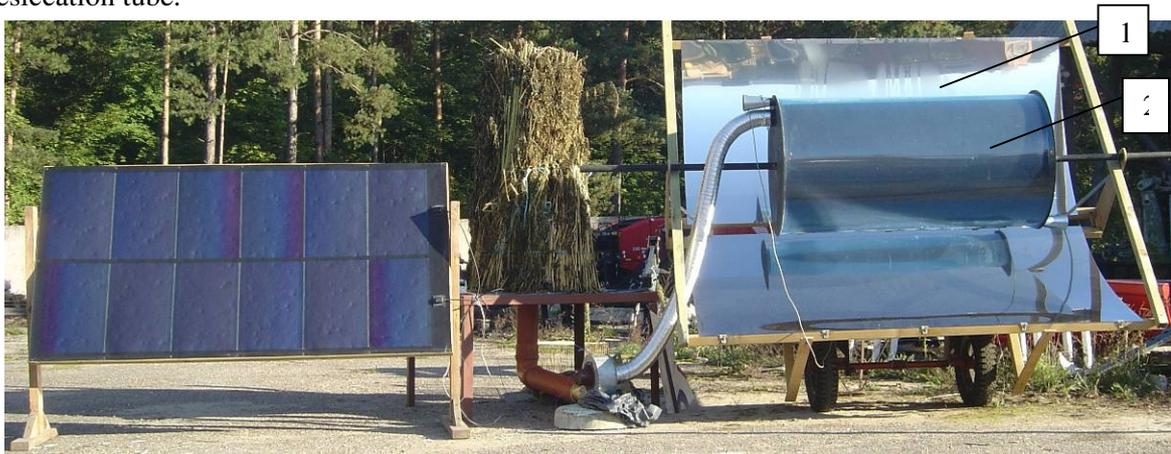
Fig. 2. Hemp desiccation device with the heated air and solar radiation energy concentrator: 1 – concentrator; 2 – heater
