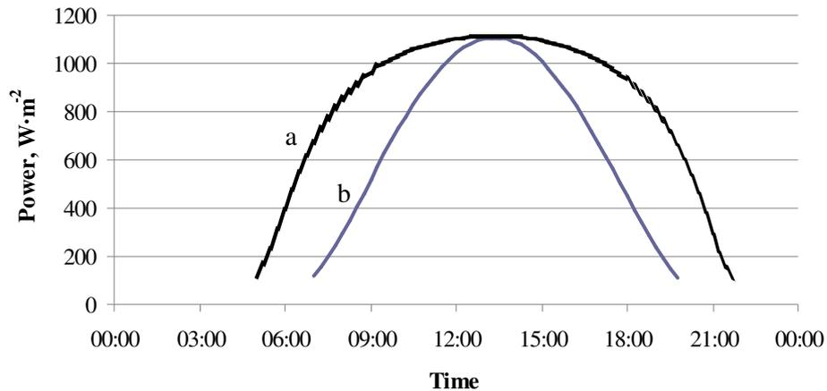
Fig. 5. Theoretically calculated daily course of power of solar collectors: a – cylindrical; b – flat
