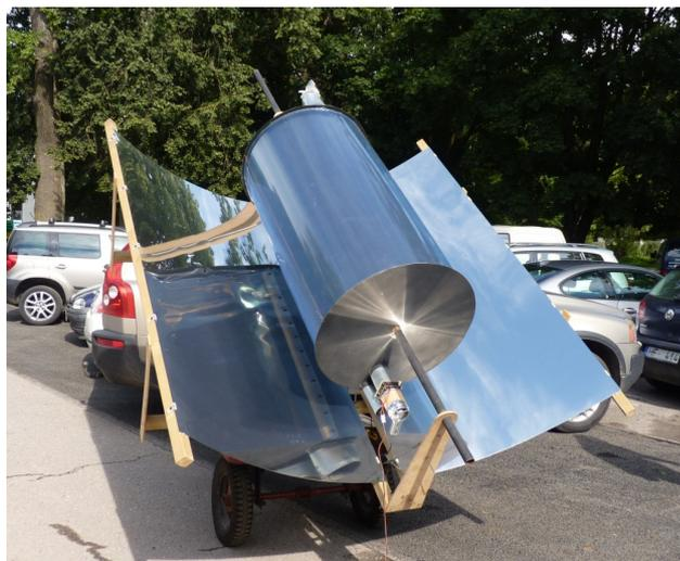
Fig. 2. Cylindrical solar collector with reflector
