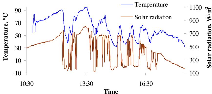
Fig. 7. Daily course of temperature of air outflowing from cylindrical solar collector with reflectors and global solar energy
