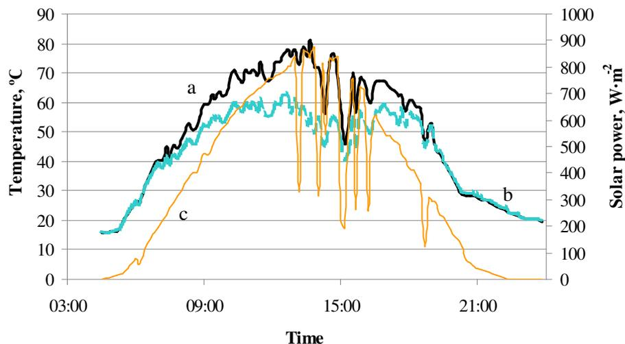
Fig. 6. Daily course of temperature of air outflowing from cylindrical solar collector (a and b) and global solar power (c)
