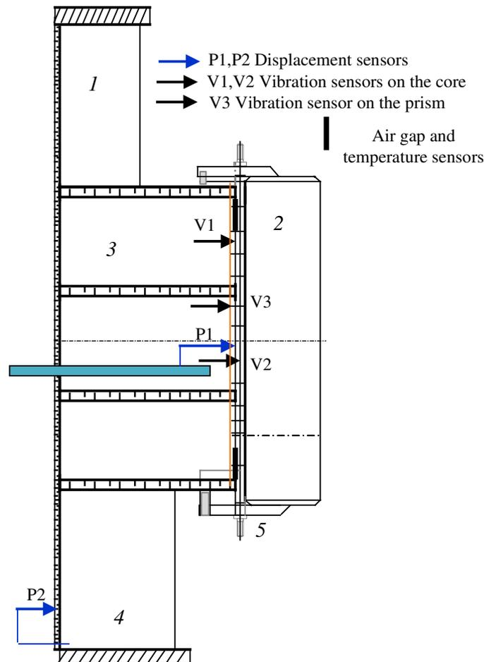
Fig. 1. **Position of the sensors for the measurement:** 1 – stator frame; 2 – stator core; 3 – openings in the shell plate for cooling air flow; 4 – sliding feet plates and foundation plates; 5 – pressure segments and non-magnetic pressure fingers
