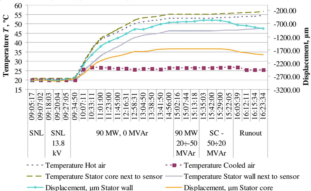
Fig. 5. Stator wall displacement depending on temperature
