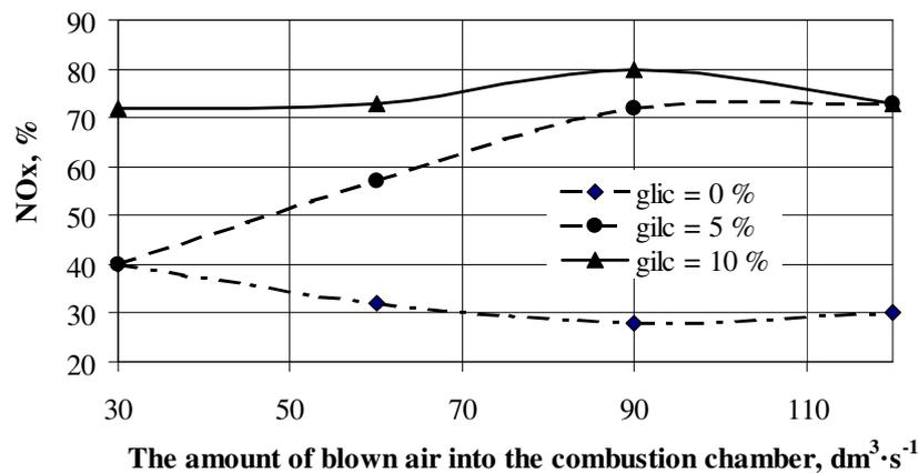
Fig. 4. Amount of NO<sub>x</sub> in the burning gases
