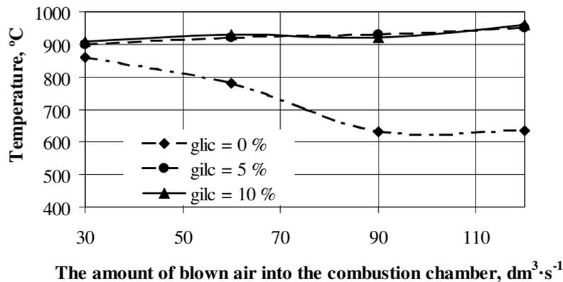
Fig. 2. Temperature in burning chamber
