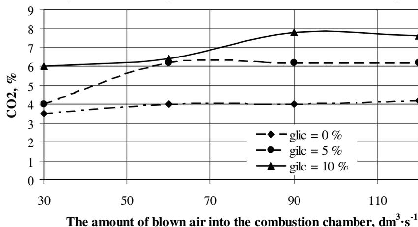
Fig. 3. Carbon dioxide in the burning gases
