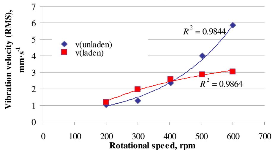
Fig. 5. Cutter head bearing housing vibration velocity (RMS) values
