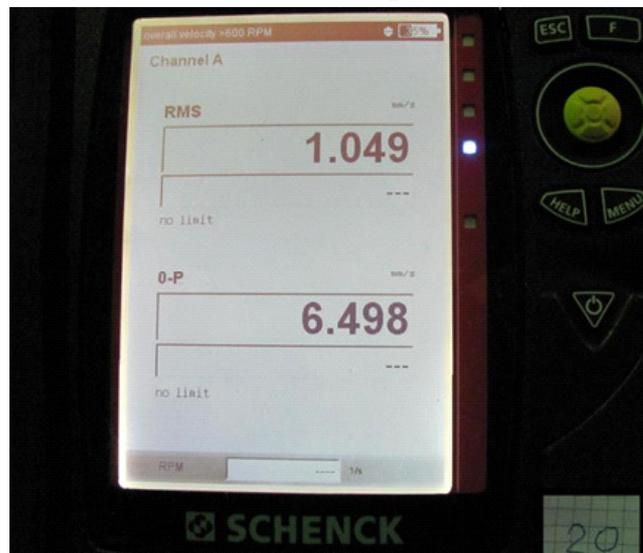
Fig. 3. Example of vibration velocity (RMS) reading
