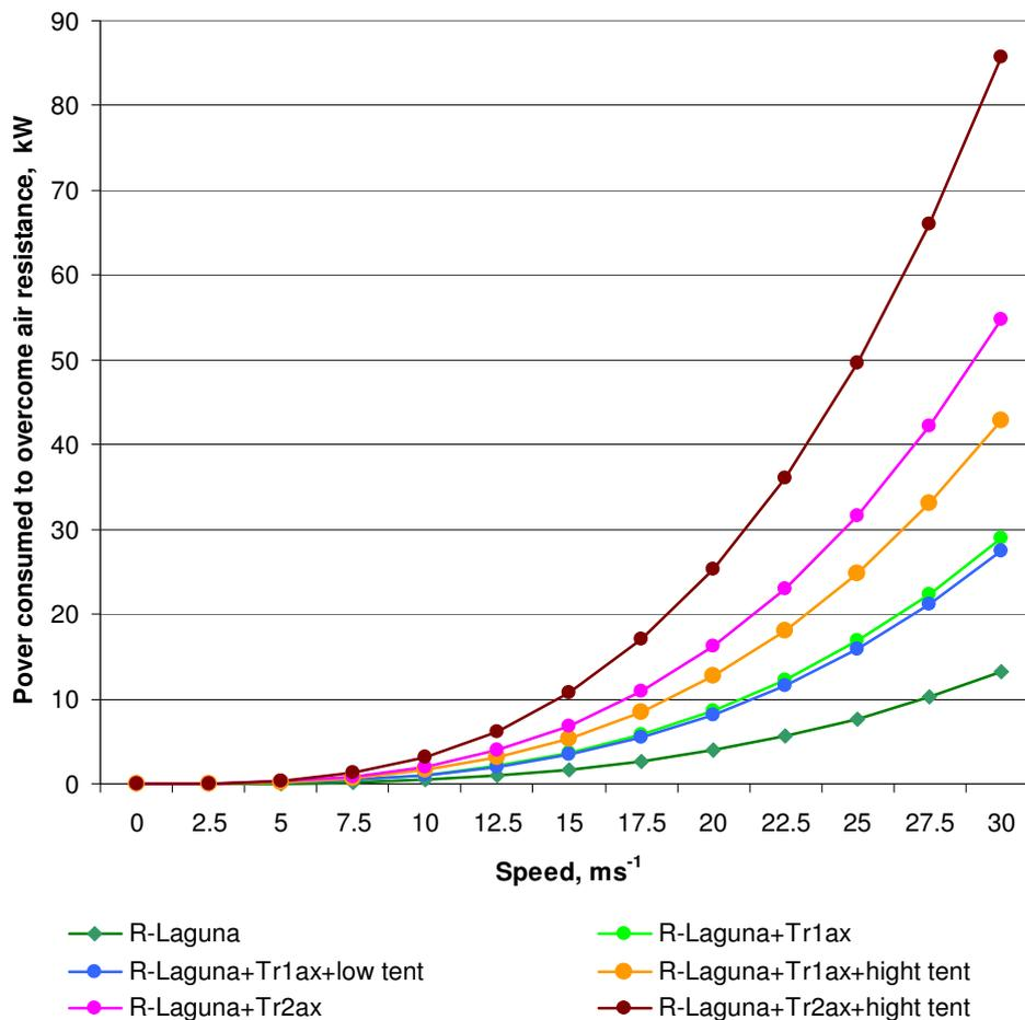
Fig. 2. Power consumed to overcome air resistance for a pulling automobile Renault Laguna
