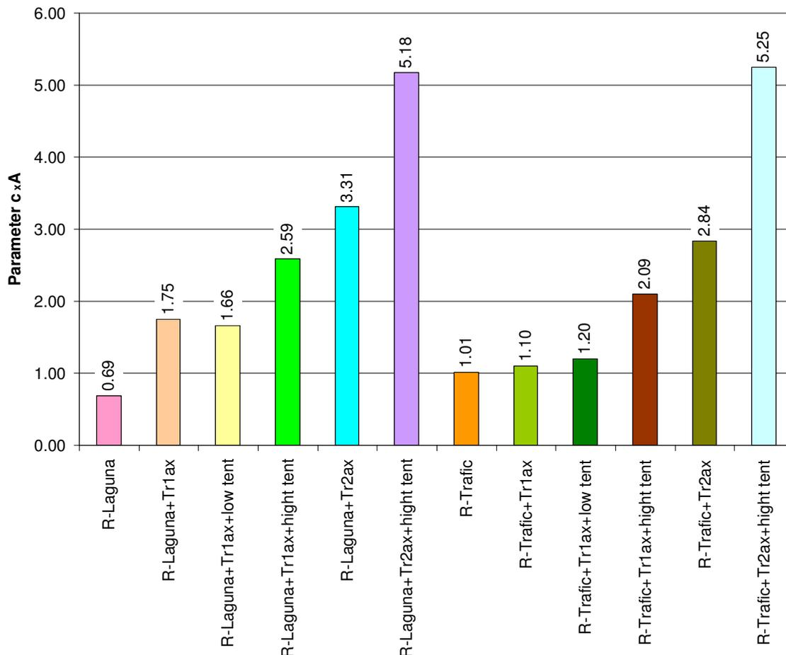
Fig. 1. Air resistance parameter  $c_xA$  for selected vehicles
