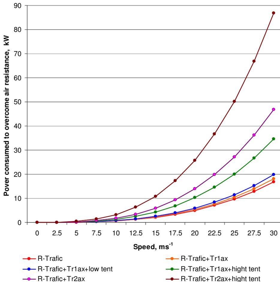
Fig.3. Power consumed to overcome air resistance for an automobile Renault Traffic
