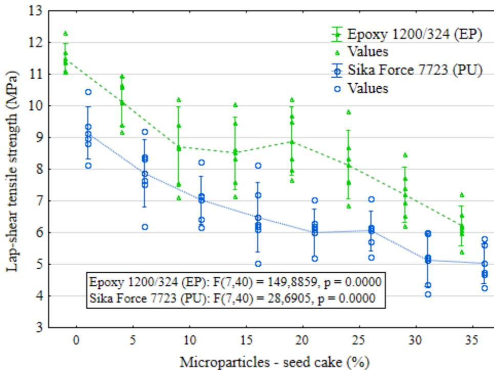
Fig. 2. Lap-shear tensile strength of composite systems
