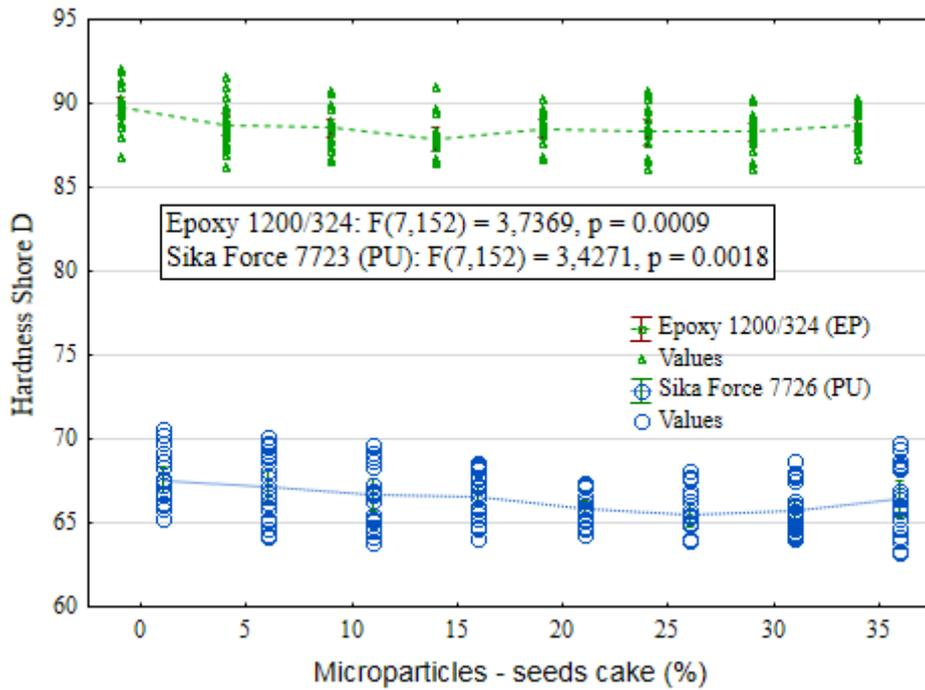
Fig. 1. Hardness Shore D of composite systems
