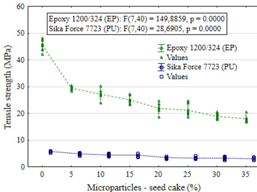
Fig. 3. Tensile strength of composite systems
