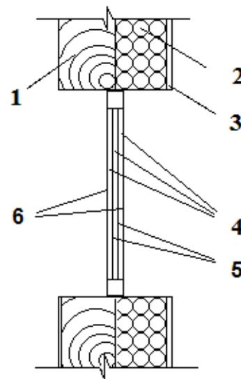
Fig. 2. Window opening with additional glasses: 1 – wood wall; 2 – polystyrene insulation; 3 – wood finish; 4 – three air gaps; 5 – original glasses of package; 6 – additional glasses
